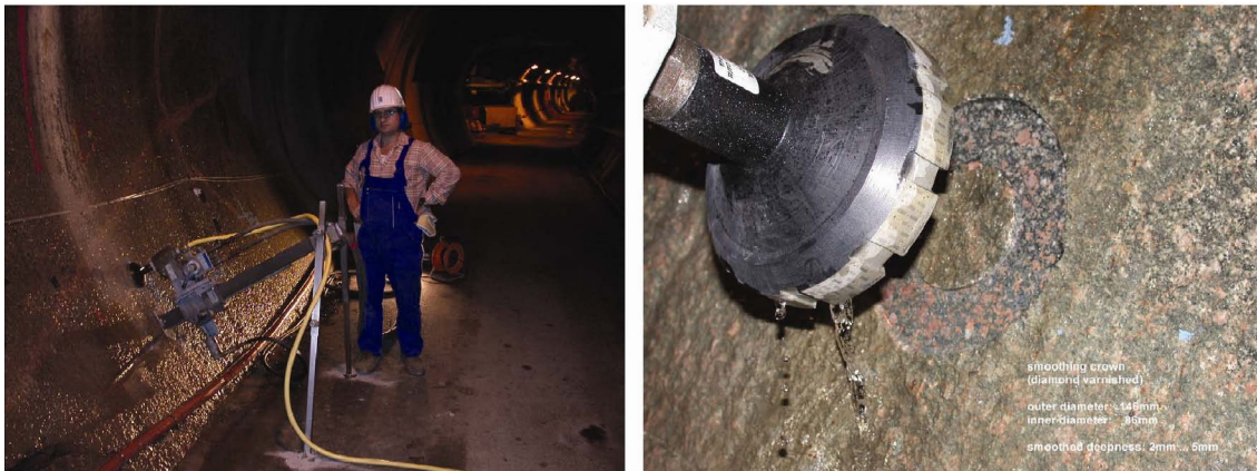
Figure 3-1. Preparation of a surface packer test location.
