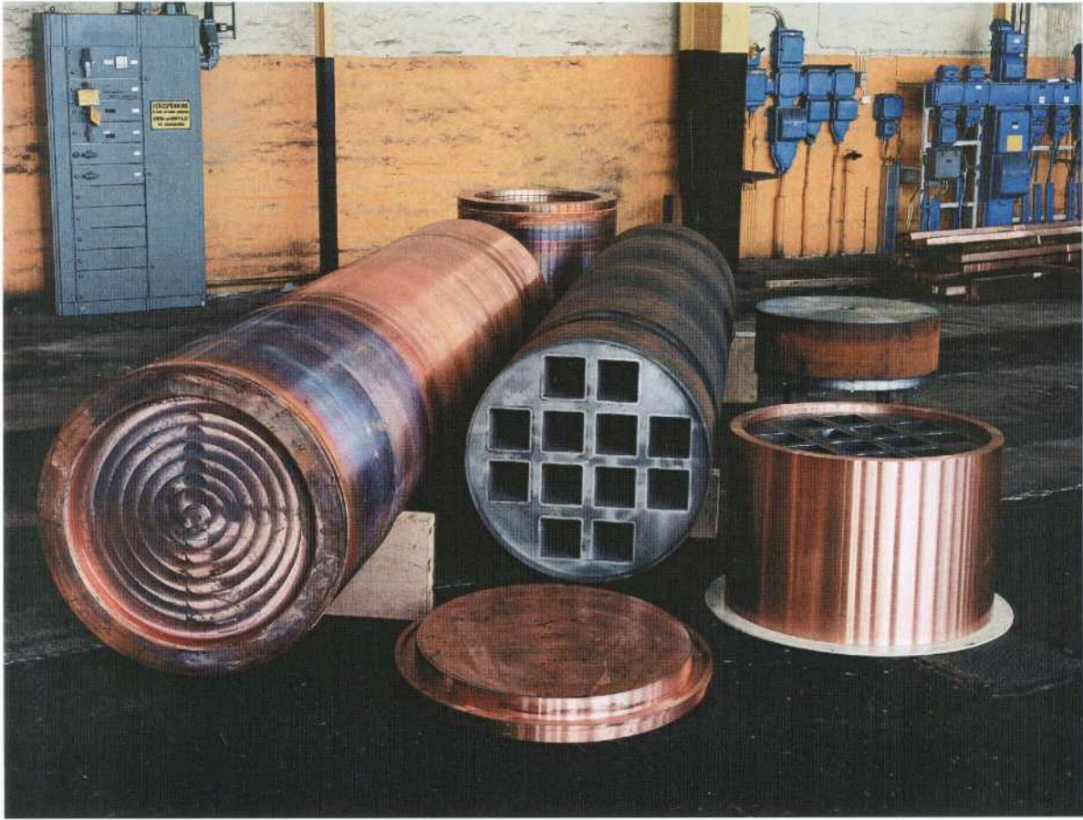
Figure 1-1. Test manufacturing of canisters. The picture shows a copper canister with a cast insert, a copper lid and some exhibits.
