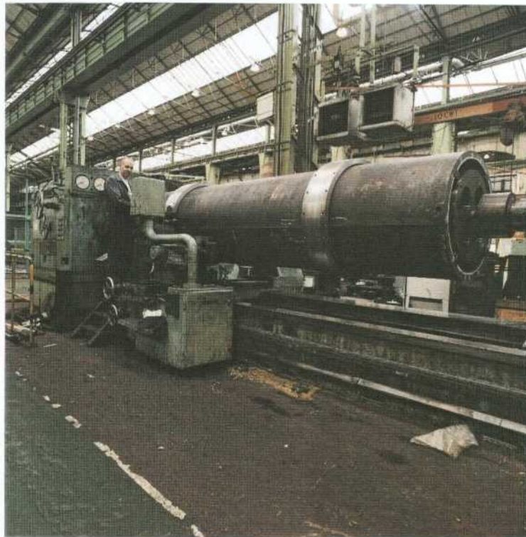
Figure 3-6. Internal drilling of a copper tube.
