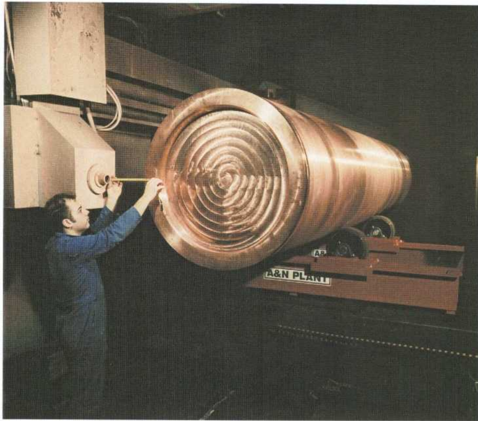
Figure 4-3. Tube T 9 in the vacuum chamber for the welding on of the bottom. The picture also shows the location of the electron gun. During the welding, the tube is rotated while the electron gun remains in a fixed position.
