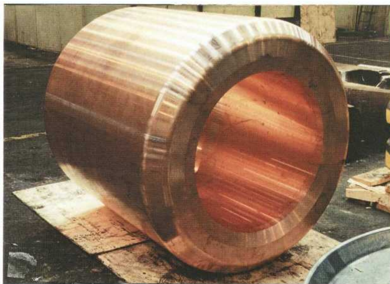
Figure 3-10. Photo of a punched blank ready for extrusion.
