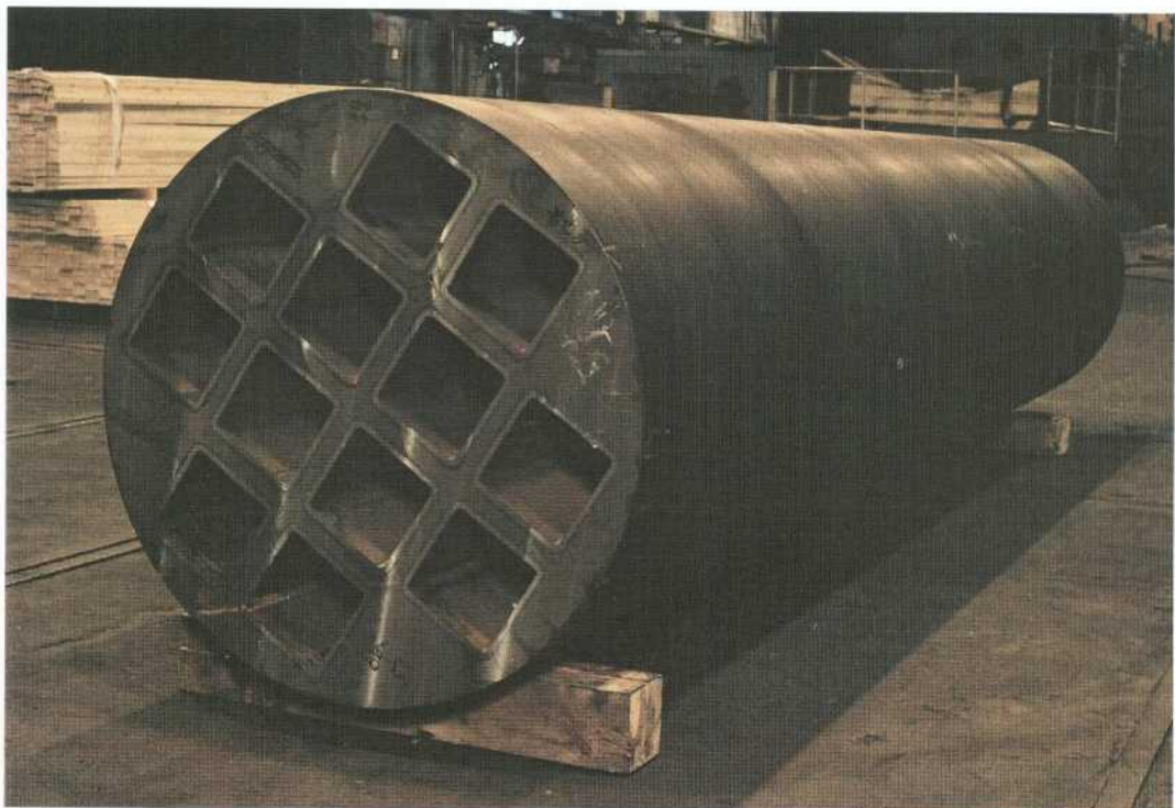
Figure 3-17. Nodular iron insert after turning of the outer surface as seen from the upper section of the insert. The machining of the top, forming the mounting for the steel lid, remains to be done.
