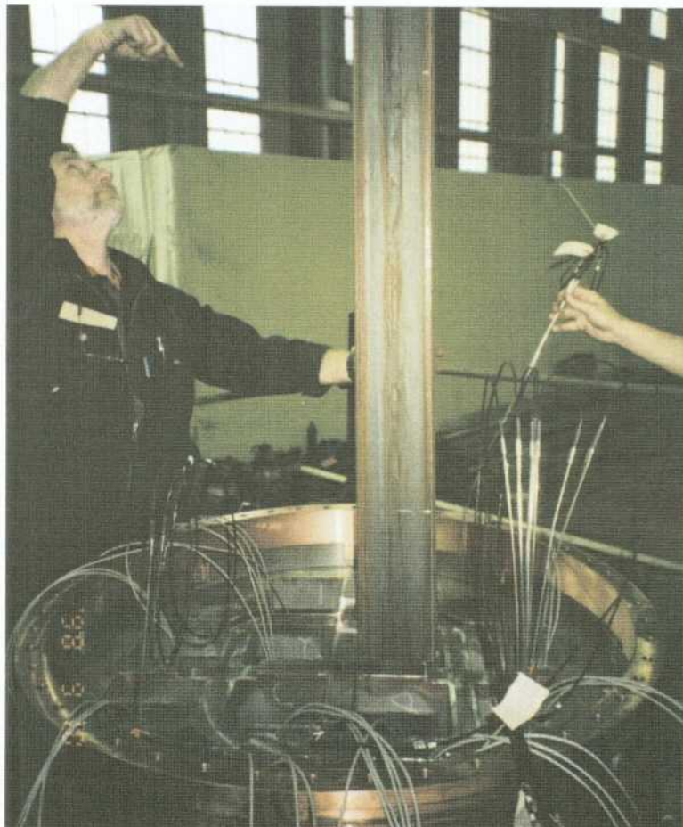
Figure 4-12. Heat elements with the same measurements as the BWR fuel assemblies, are placed in the channels of the insert. The canister is equipped with a number of thermal elements both internally and externally.
