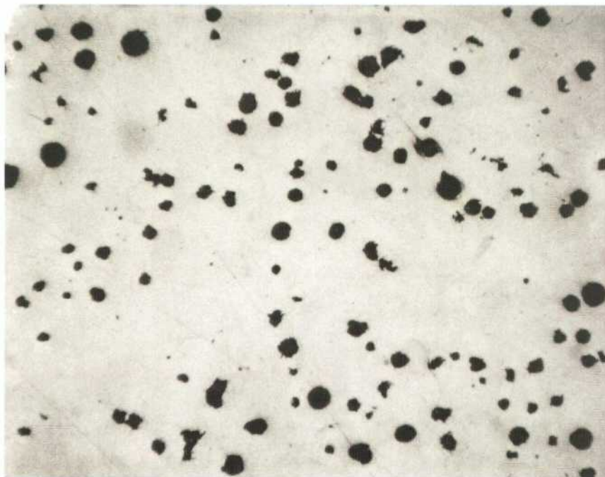
Figure 4-8. The structure in a tensile testing bar for insert I 7, cast in the same test. Etched 2% Nital. (100x)
