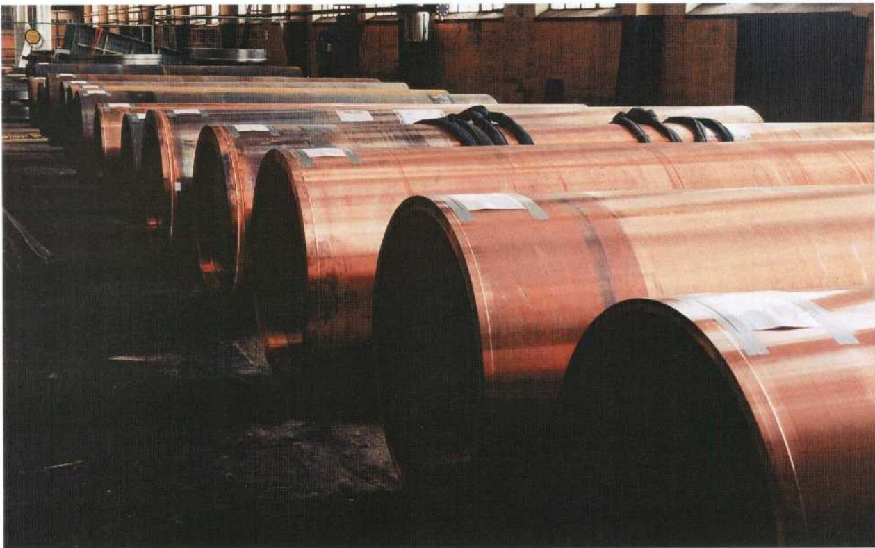
Figure 1-2. Test manufacturing of canisters. The picture shows copper tubes and inserts. Two of the copper inserts have welded-on bottoms.
