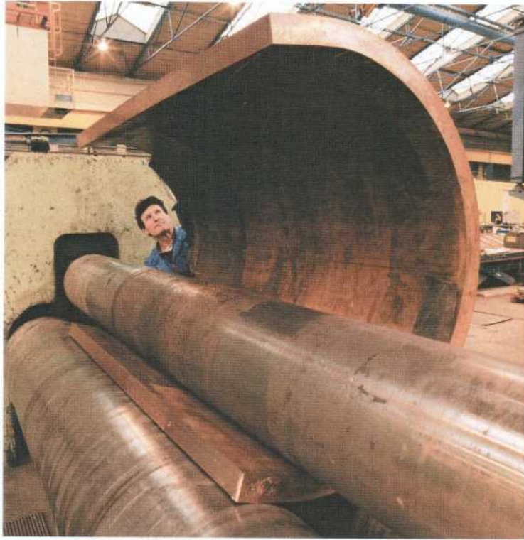
Figure 3-1. Roll-forming of a short copper tube.
