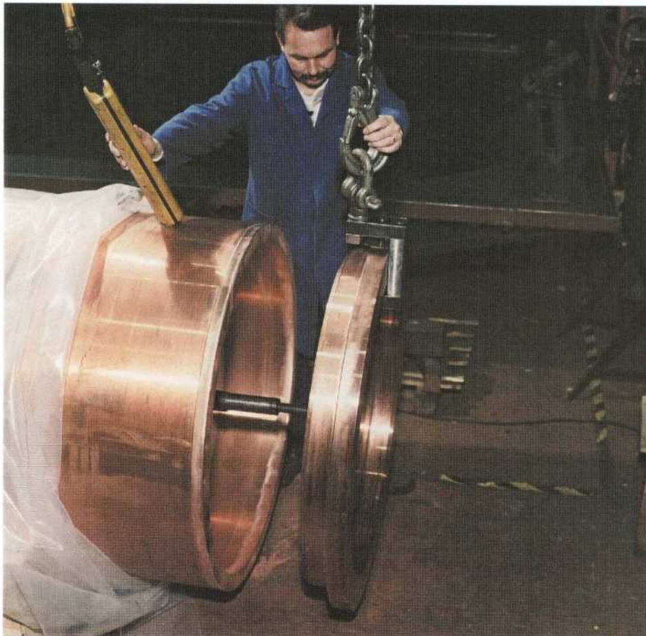
Figure 4-2. The fitting of the bottom onto tube T 9.
