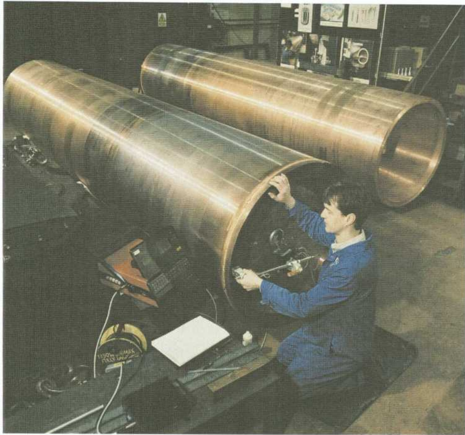
Figure 4-4. Ultrasound examination (P-scanning) of the bottom weld on TB 3/T 9.
