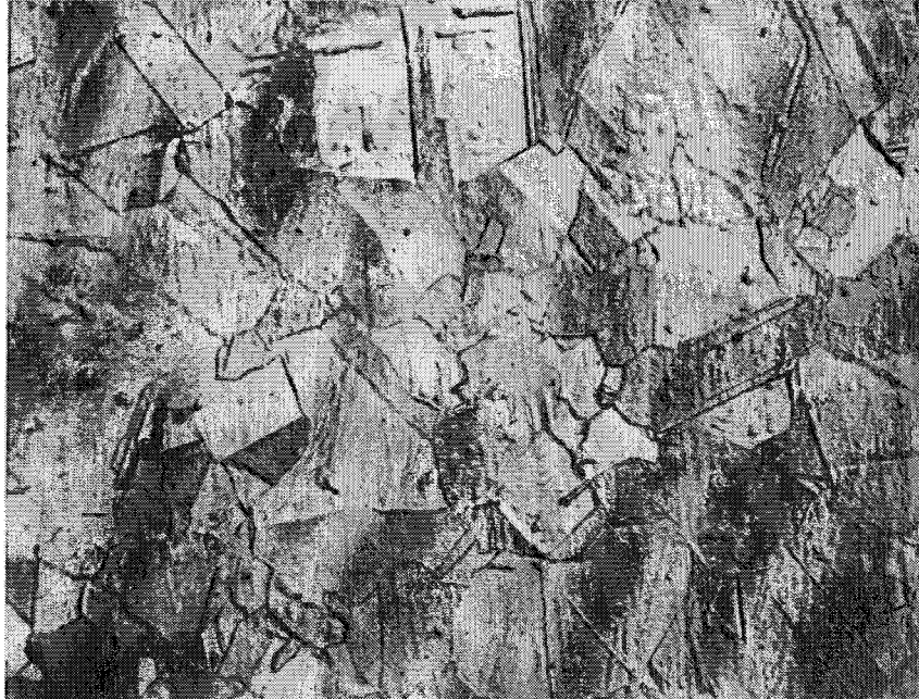
Figure 4-1. The structure in the top section of the T 21 tube. 100x.
