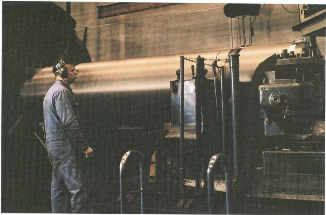
Figure 3-16. Turning of cast insert in nodular iron.
