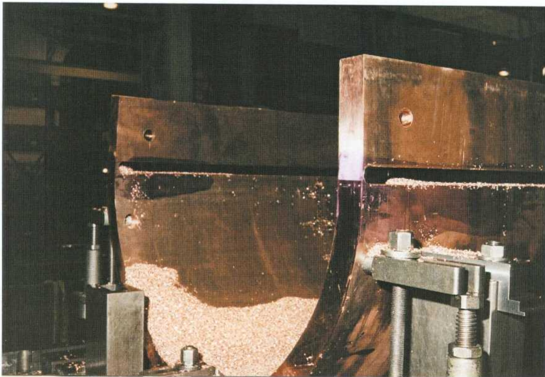
Figure 3-3. Machining of surplus measurement on roll-formed tube halves.
