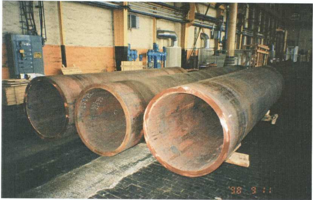
Figure 3-12. Extrusion-processed copper tubes. As with pierce and draw processing, the last stage in the manufacturing of copper tubes using this method, is the inner and outer machining.
