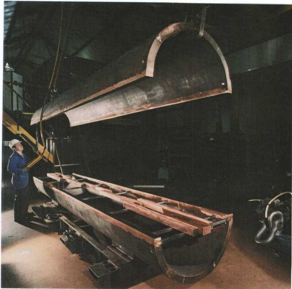
Figure 3-4. The putting together of tube halves for electron beam welding. The copper bars in the middle have been placed there in order to prevent the opposite wall from being hit by the electron beam during the longitudinal welding.
