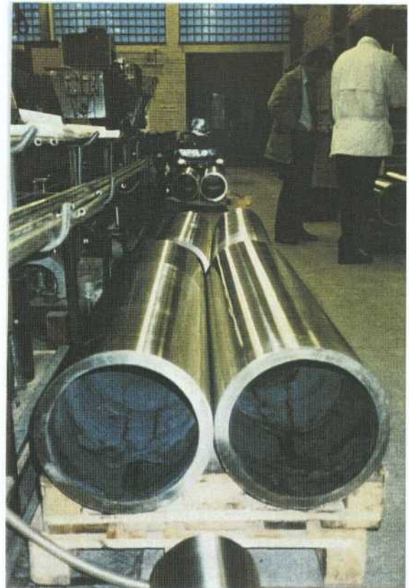
Figure 5-2. Manufacturing of tubes using the Osprey process.
