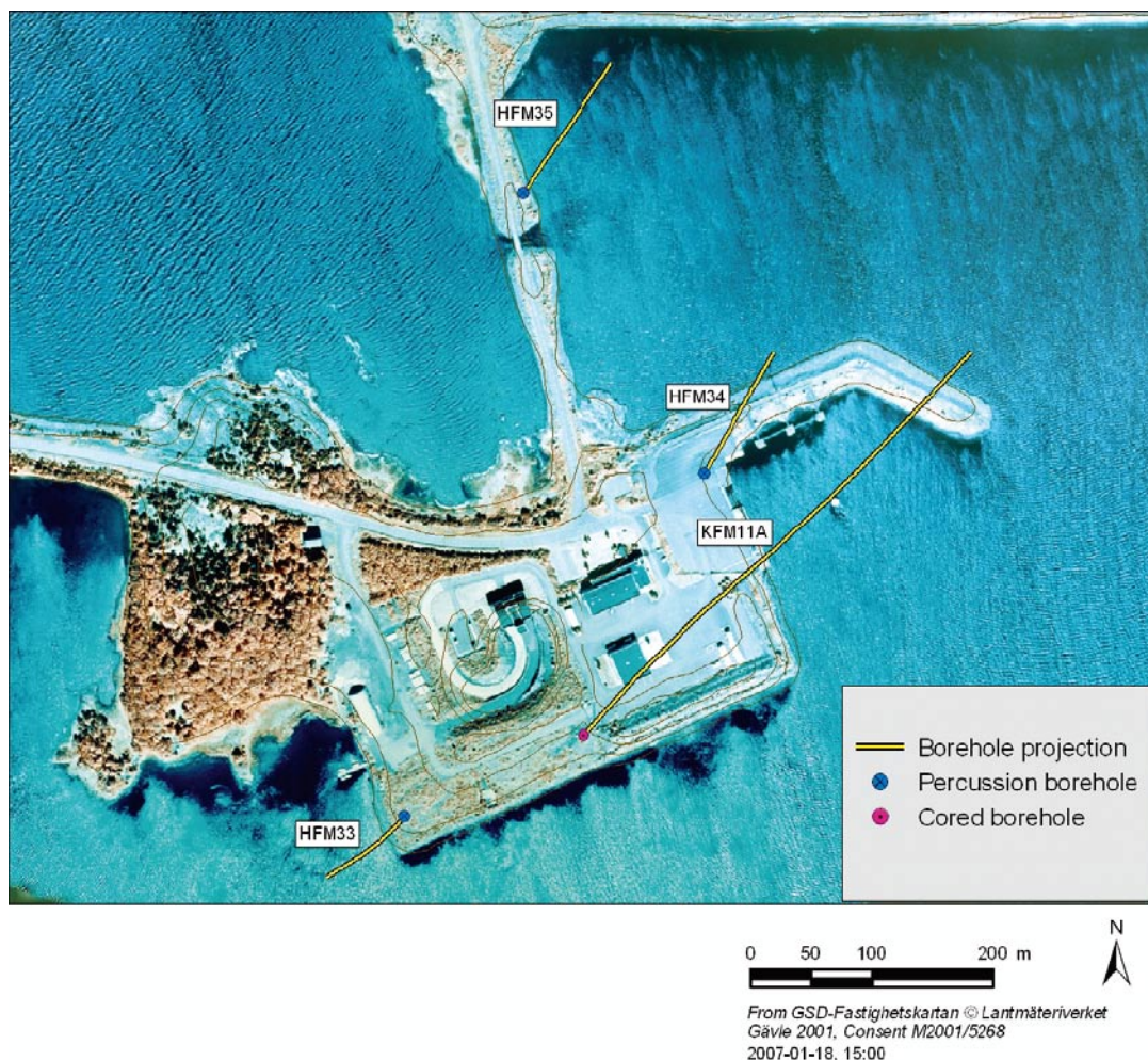
Figure 1-2. Borehole locations at and near drill site DS11. Besides the core drilled borehole KFM11A, the area incorporates a flushing water well (HFM33), and two monitoring wells in bedrock (HFM34-35). Also HFM33 will later be used as a monitoring well. The projection of inclined boreholes on the horizontal plane at the ground surface (top of casing) is shown in the figure.
