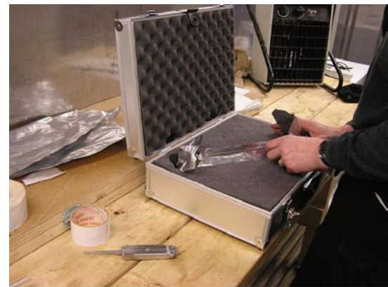
Figure 5-9. The photos show the careful handling of the samples for pore space groundwater in low permeable rock performed in KFM01D. The same procedure was applied in KFM02B. To the upper left the core has been recovered from the borehole and is placed in a nitrogen filled plastic bag from which the nitrogen is evacuated. To the upper right the plastic bag is permanently heat sealed. To the lower left the sample is well preserved in two plastic bags and a third plastic bag lined with aluminium foil is also permanently heat sealed. Finally, to the lower right, the sample is placed in a shock proofed aluminium box that within 24 hours is delivered to the University of Bern.
