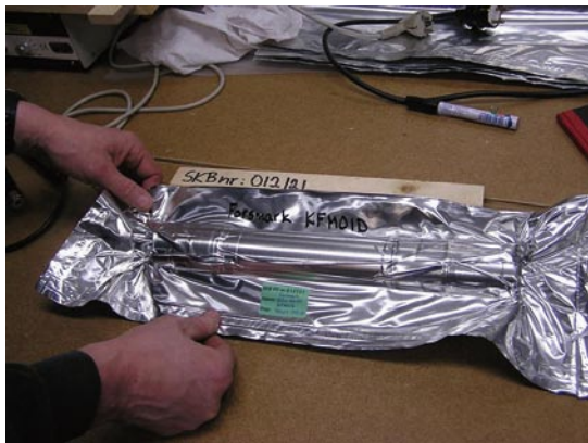
Figure 5-9. The photos show the careful handling of the samples for pore space groundwater in low permeable rock performed in KFM01D. The same procedure was applied in KFM02B. To the upper left the core has been recovered from the borehole and is placed in a nitrogen filled plastic bag from which the nitrogen is evacuated. To the upper right the plastic bag is permanently heat sealed. To the lower left the sample is well preserved in two plastic bags and a third plastic bag lined with aluminium foil is also permanently heat sealed. Finally, to the lower right, the sample is placed in a shock proofed aluminium box that within 24 hours is delivered to the University of Bern.
