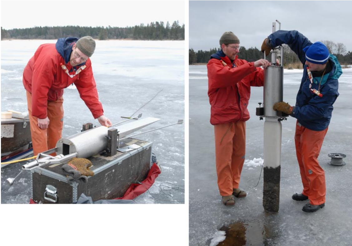
Figure 3-2. Freeze corer, before use (left), with sample (right).
