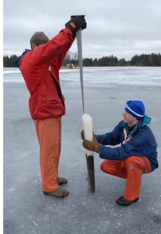
Figure 3-3. Detaching of the sediment sample. 1) Poring hot water into the freezing wedge (left), 2) lifting out the wedge (right).
