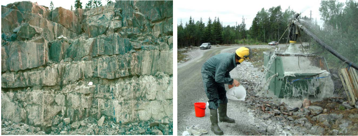
Figure 4-29. Two pictures of the near-surface bedrock in the north-western part of the tectonic lens (target area). The leftmost picture shows structurally dominant, but highly heterogeneous, horizontal sheet joints where the apertures are clogged by glaciofluvial sediments. This phenomenon is known to occur down to at least c. 50 m depth (KFM03A and HFM07) rightmost picture shows the flushing of a high yielding gently dipping deformation zone or sheet joint encountered at c. 40 m depth in HFM02.
