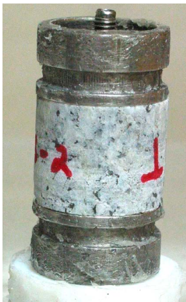
Figure 4-4. Rock core sample enclosed by end pieces to be used in a permeability measurement. Reproduced from /Vilks 2007/.
