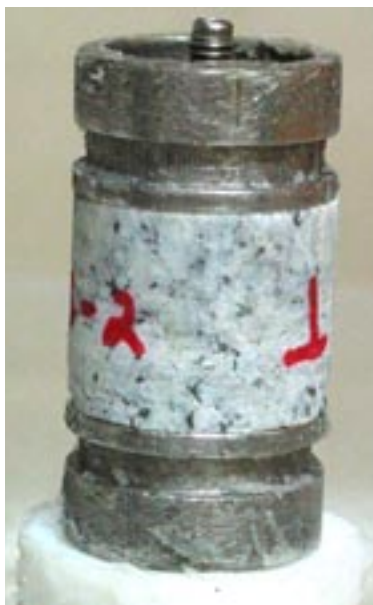
Figure 4-4. Rock core sample enclosed by end pieces to be used in a permeability measurement. Reproduced from /Wilks 2007/.
