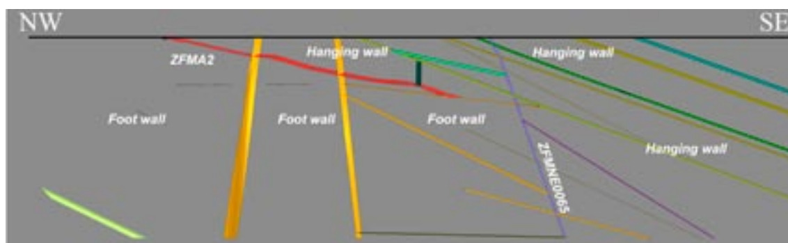
Figure 8-1. Cross section of the deformation model. The profile is circa six kilometres long and two kilometres deep. Modified after /Stephens et al. 2007/.
