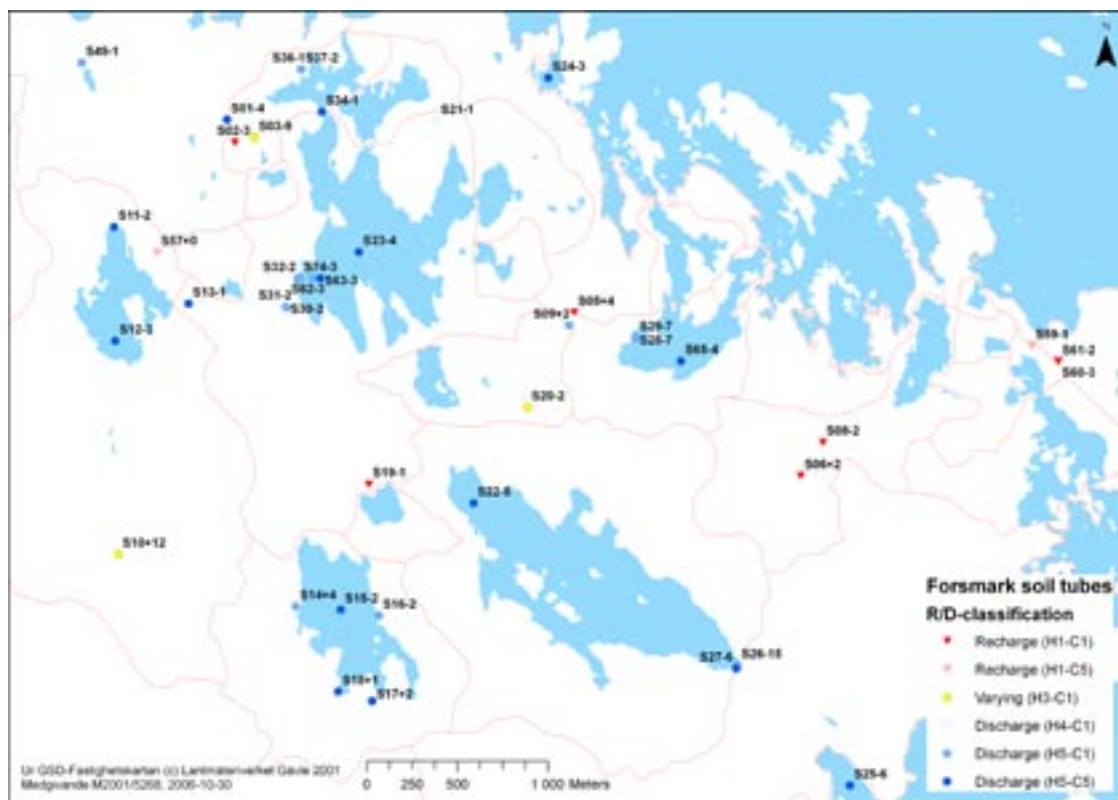
Figure 5-10. Map showing the geographical distribution of soil tubes according to the six available combinations in Table 5-2. “H” denotes hydrological class and “C” chemical class.
