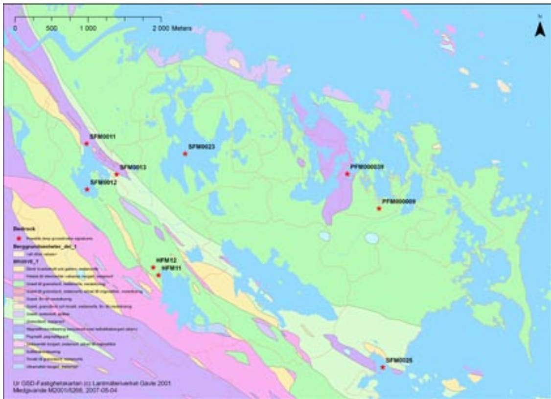
Figure 4-21. Shallow groundwater objects (soil tubes and drilled private wells) that show possible deep groundwater signatures. See Table 4-2 for an explanation of individual objects. Two percussion drilled boreholes, HFM11 and HFM12, have also been included as they show the strongest shield brine signatures among all percussion drilled boreholes in the upper part of the bedrock.
