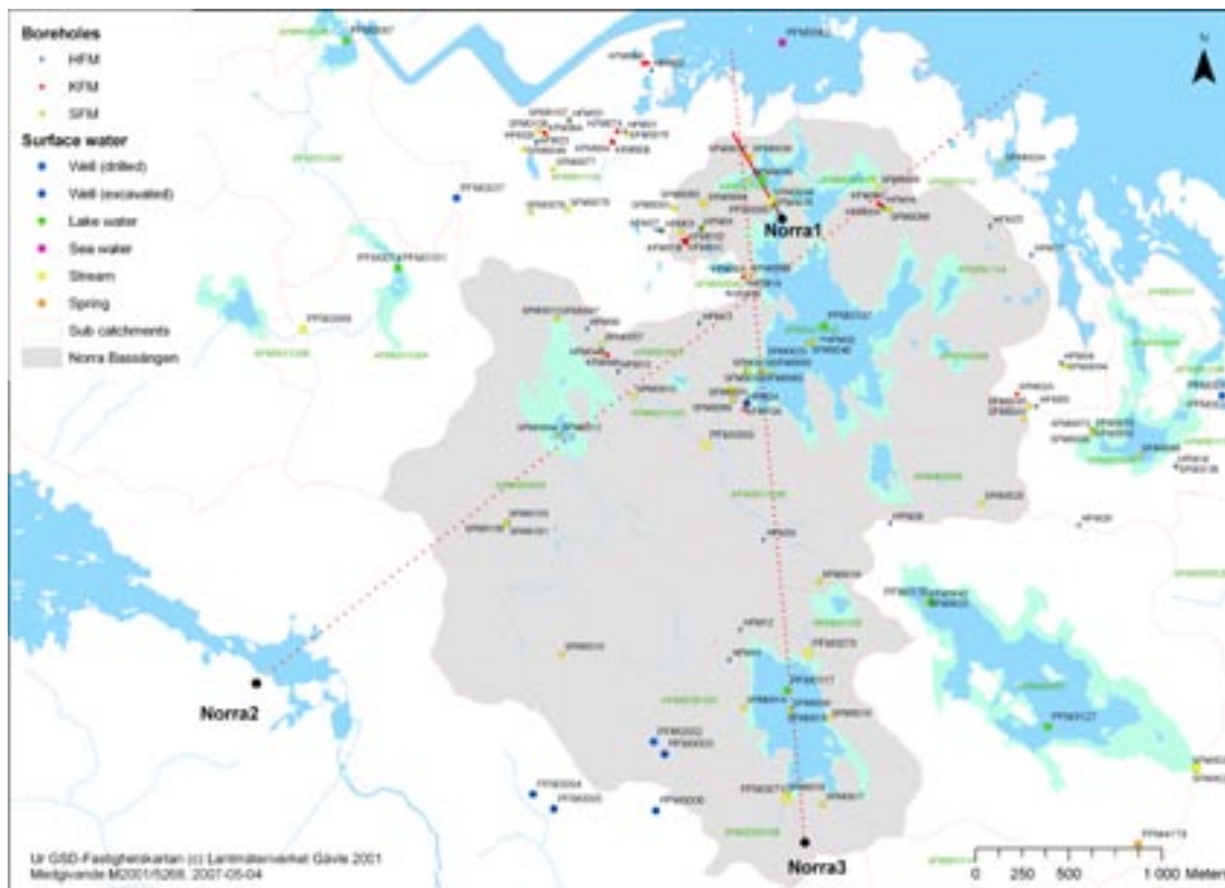
Figure 7-14. The catchment of Norra Bassängen. Red dotted lines denote the location of vertical profiles showing cross sections including soil layers, groundwater levels and boreholes in the vicinity of these transects (profiles start at the end marked with a black dot). Boreholes within a specified distance from the transects are included in the profile plots (Norra 1: 100 m, Norra 2: 700 m, Norra 3: 500 m respectively).
