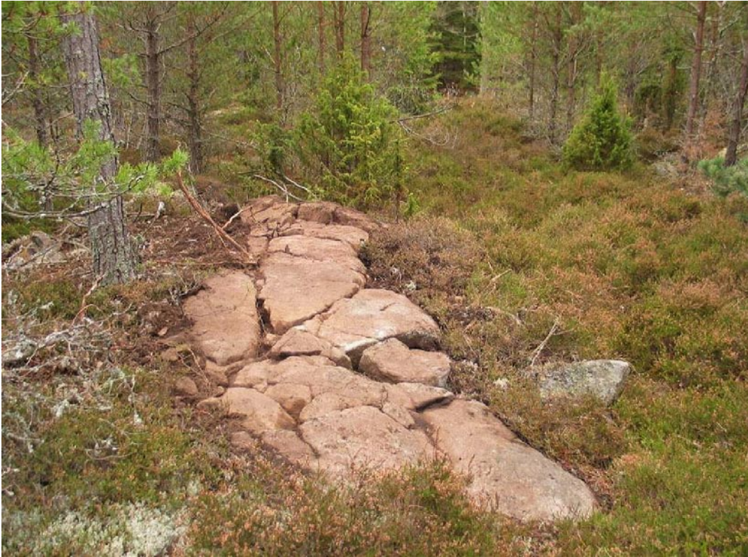
Figure 4-31. At outcrop A11 part of the deformation zone width was uncovered in two locations a few metres apart, Appendix A. The rock is here strongly affected by cataclastic deformation, in what is best described as a brittle-ductile deformation zone. The deformed rock seems to be primarily granite, but extensive intrusion of brecciating quartz and intensive alteration and fracturing make it difficult to exclude that other rock types also are involved. As can be seen in the image, the fracture frequency is high. Since the full zone width is not exposed the fracture geometries and zone geometry has not been examined.
