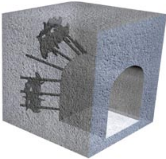
Figure 3-2. Illustration of a part of a grouting fan in a tunnel. The boreholes that intersect conductive fractures contribute to the sealing effect. After /Eriksson and Stille 2005/.
