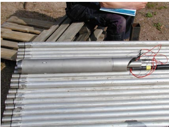
Photo 5. Positioner, bottom end of down-in-hole string.
