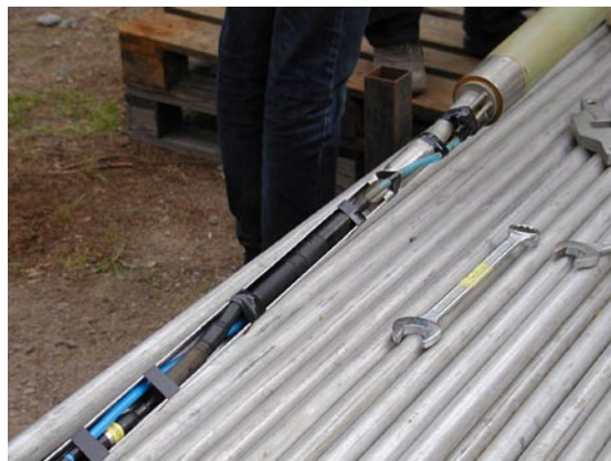
Photo 6. Packer and gauge carrier.
