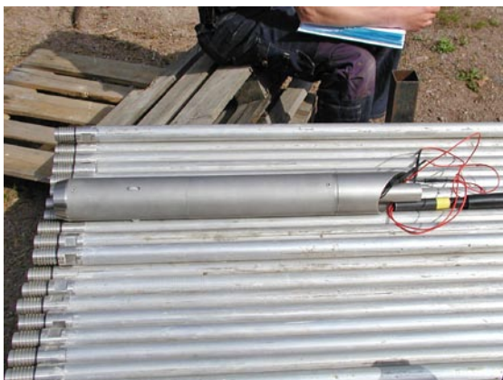
Photo 5. Positioner, bottom end of down-in-hole string.
