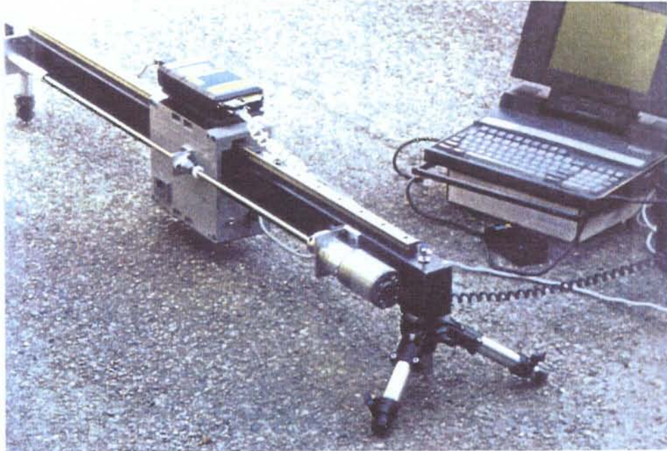
Figure 6.1-1. The optical linear laser profilometer (Halttunen 1995).
