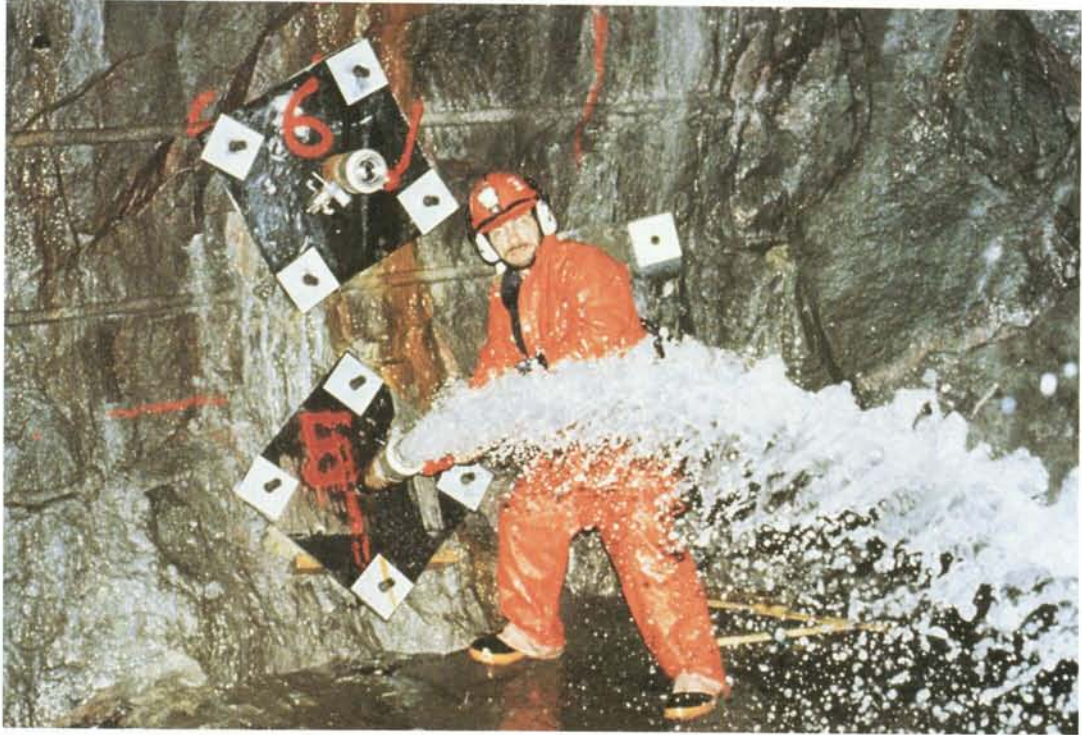
Figure 1-10. When the valve on the casing was opened about 1600 litres per minute flowed out of a borehole (with a diameter 57 mm) drilled into the structure NE-1 (below the Baltic sea).
