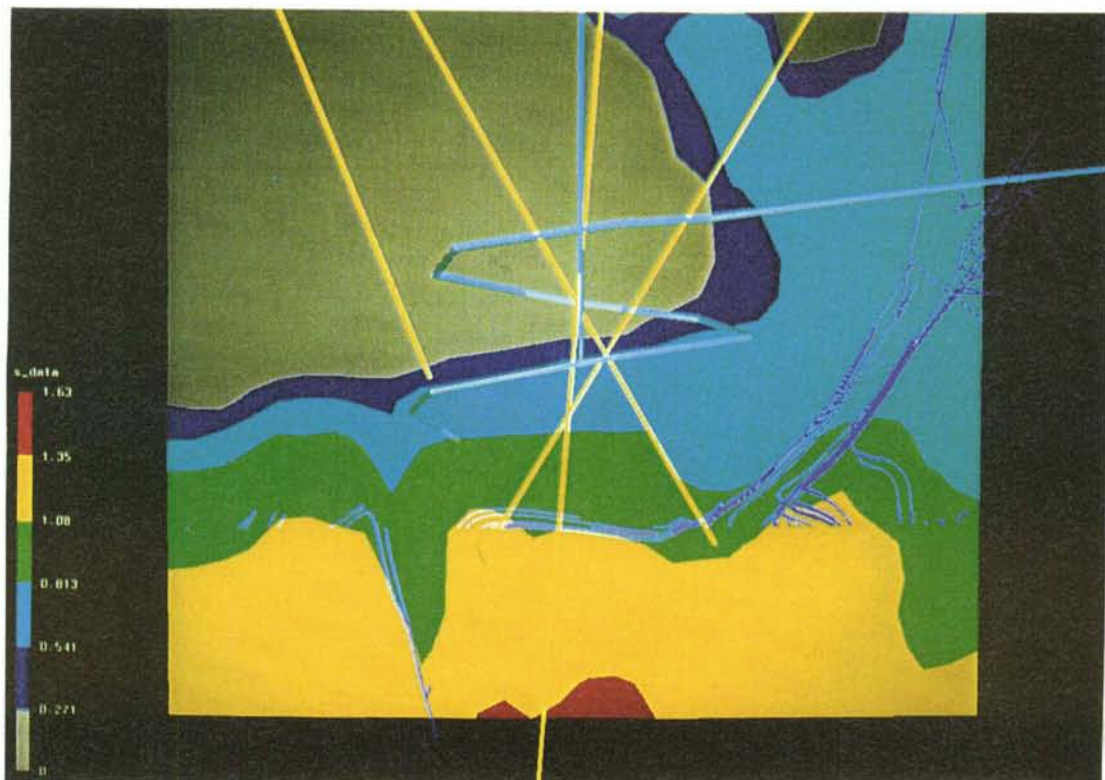
Figure 2-8. Construction phase, TFP = 1475 m - Numerical groundwater flow simulations. Hydraulic conductor domain NNW-4, view from west. Top: Flow and pressure, with the hydrostatic component \rho_0 g subtracted ( \rho_0 = 1000 \text{ kg/m}^3 ). Bottom: Salinity and some stream lines.
