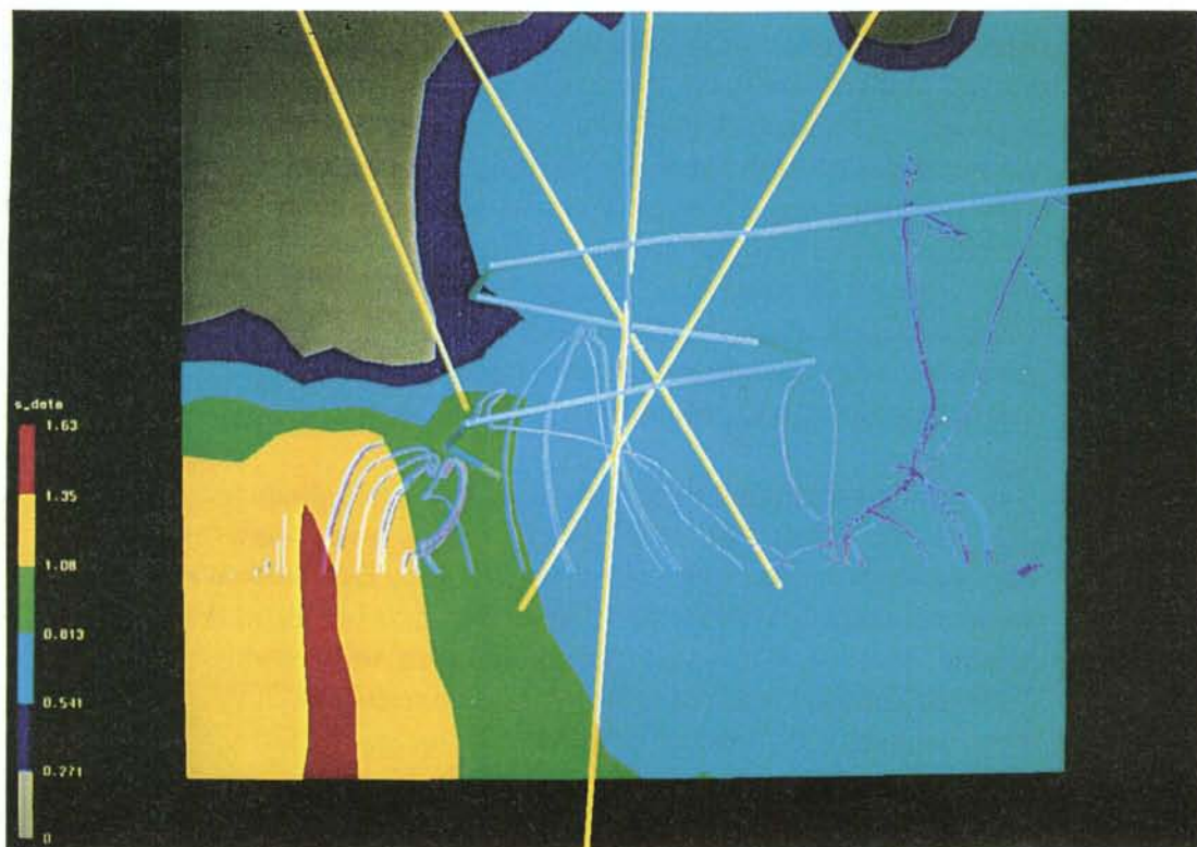
Figure 2-9. Construction phase, TFP = 2874 m - Numerical groundwater flow simulations. Hydraulic conductor domain NNW-4, view from west. Top: Flow and pressure, with the hydrostatic component \rho_0 g subtracted ( \rho_0 = 1000 \text{ kg/m}^3 ). Bottom: Salinity and some stream lines.
