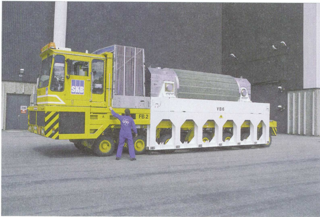
Figure 6-5. Transport cask during transport on terminal vehicle. The cask is of the type that is used today for shipments of spent nuclear fuel from the nuclear power plants to CLAB.
