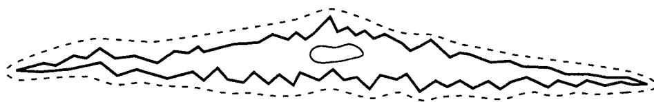
Figure 2.3 Cross-section of a fracture with actual surface of fracture (solid line) and surface as seen by a radionuclide diffused some depth into the matrix (dashed line).
