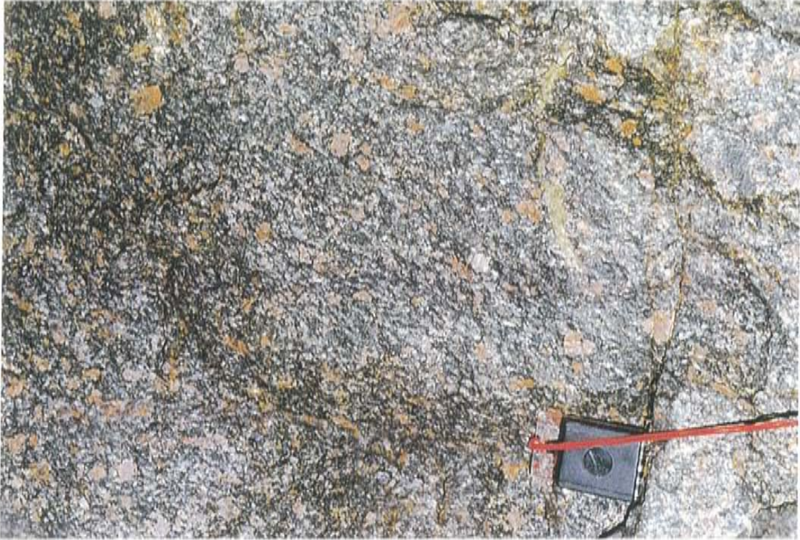
Figure 4-5. Reddish grey 'Äspö diorite' with large, scattered megacrysts of potassium feldspar. Äspö, access ramp 1770 m, photo Kristian Annertz in Wikman and Kornfält /1995/.
