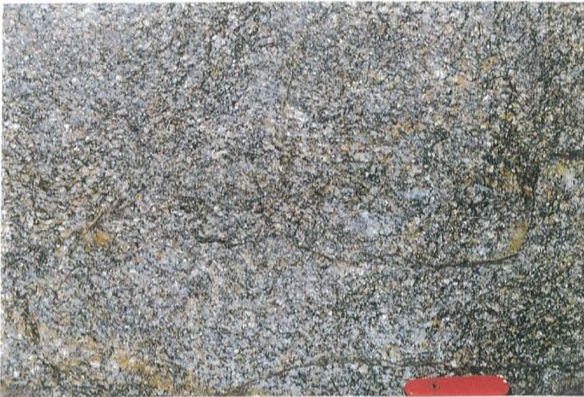
Figure 4-6. Light reddish grey Småland (Ävrö) granite. Äspö, access ramp 1775 m, photo Kristian Annertz in Wikman and Kornfält /1995/.
