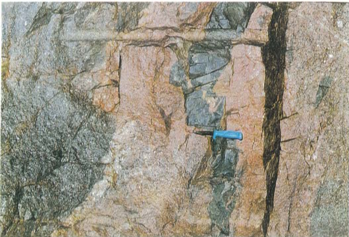
Figure 4-8. Composite dike with a fine-grained greenstone in the centre boarded by fine-grained granite. Äspö, access ramp 2193 m, photo Kristian Annertz in Wikman and Kornfält /1995/.
