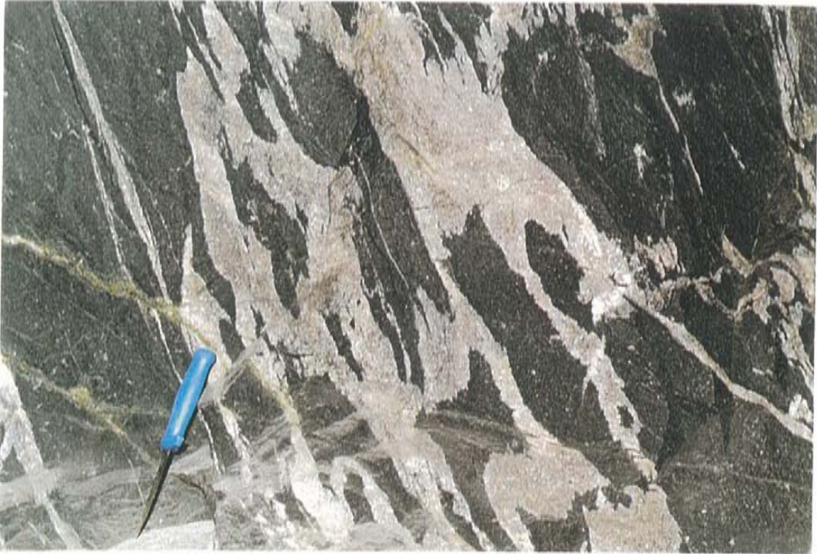
Figure 4-7. Greyish black, fine-grained greenstone intruded by fine-grained granite. Äspö, access ramp 3040 m, photo Kristian Annertz in Wikman and Kornfält /1995/.
