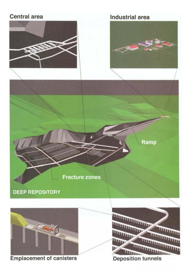
Figure 2-1. Schematic diagram of the layout of the deep repository.
