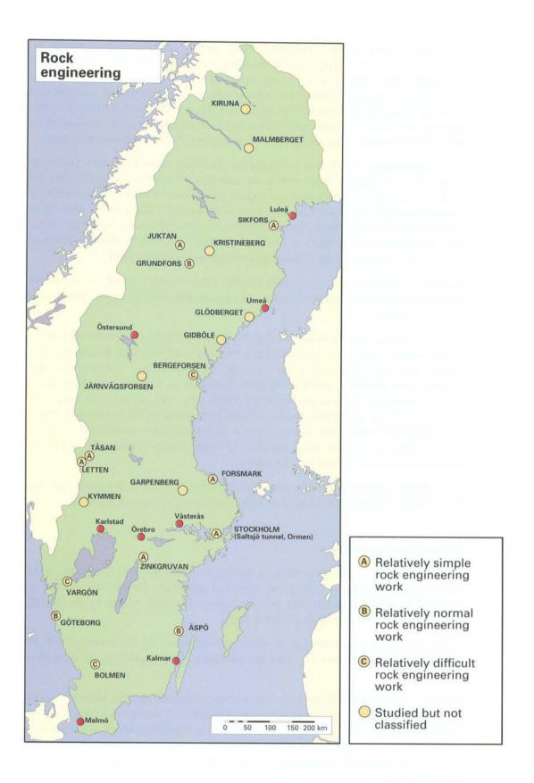
*Figure 5-10.* Rock engineering evaluated according to constructability. Based on /5-6/. The rock engineering work is determined by local factors which are investigated in feasibility studies and site investigations.
