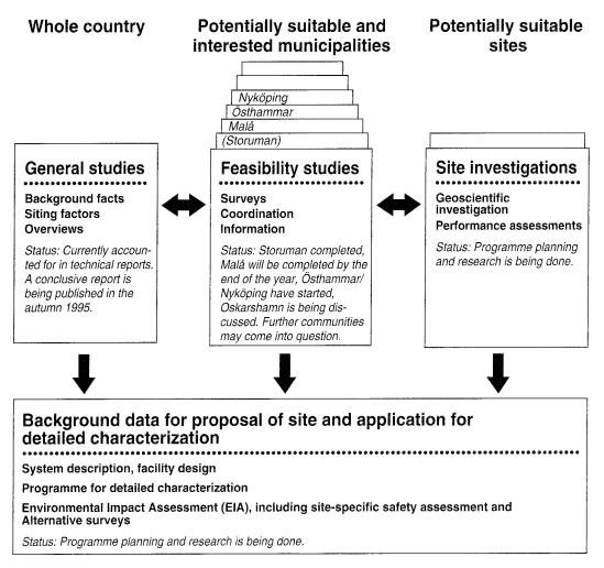
Figure 1-1. Main components of the siting work. From /1-5/.
