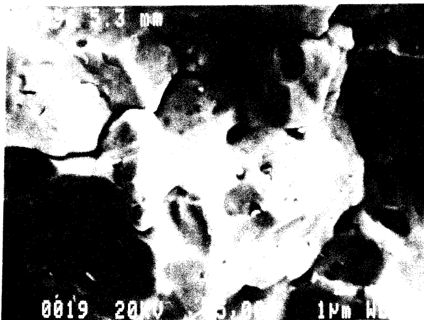
Figure 2-14. BWR fuel: (Burnup 49.0 MWd/kgU) 4d metallic particles near the pellet centre. (x 5000)
