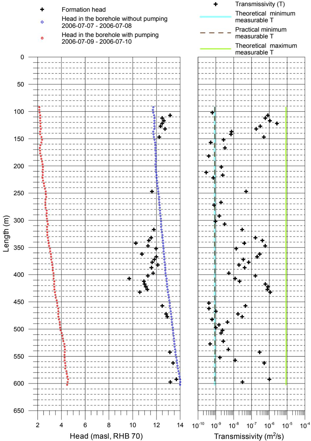
Plotted transmissivity and head of detected fractures
