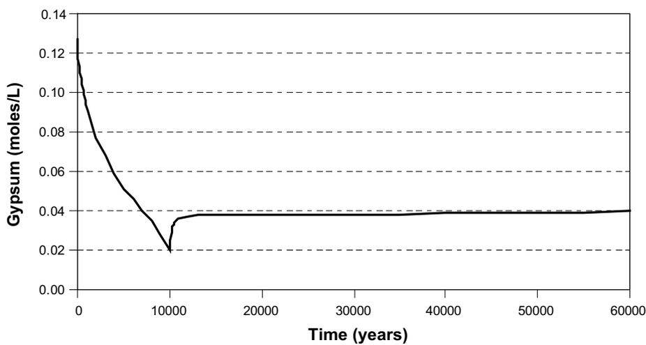
**Figure 5-22.** Predicted evolution of the gypsum content in the bentonite close to the fracture (exact location as in Figure 5-7) after the intrusion of high-salinity water.
