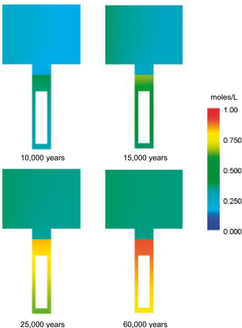
**Figure 5-54.** Predicted calcium occupancy in the exchanger of the bentonite due to the intrusion of high-salinity groundwater.
