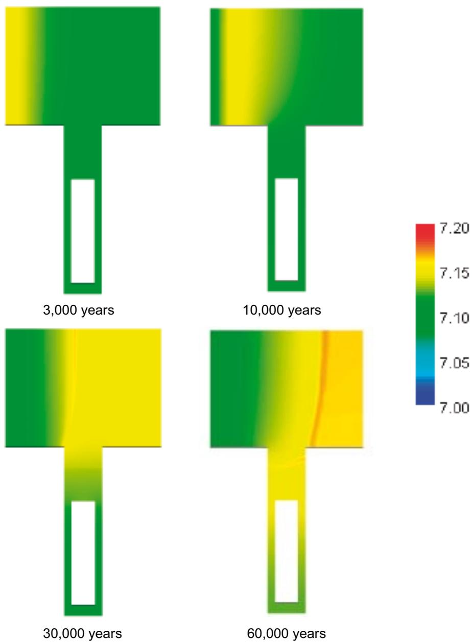
**Figure 5-56.** Predicted pH evolution due to the interaction of Forsmark groundwater with Deponit CA-N bentonite in the buffer and in the 30/70 backfill.
