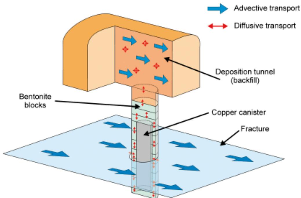
**Figure 4-1.** Schematic view of the near field of a KBS-3 repository showing the transport mechanisms in the different parts of the system.
