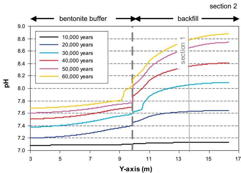
**Figure 5-61.** Predicted pH evolution due to the intrusion of ice-melting water in section 2.
