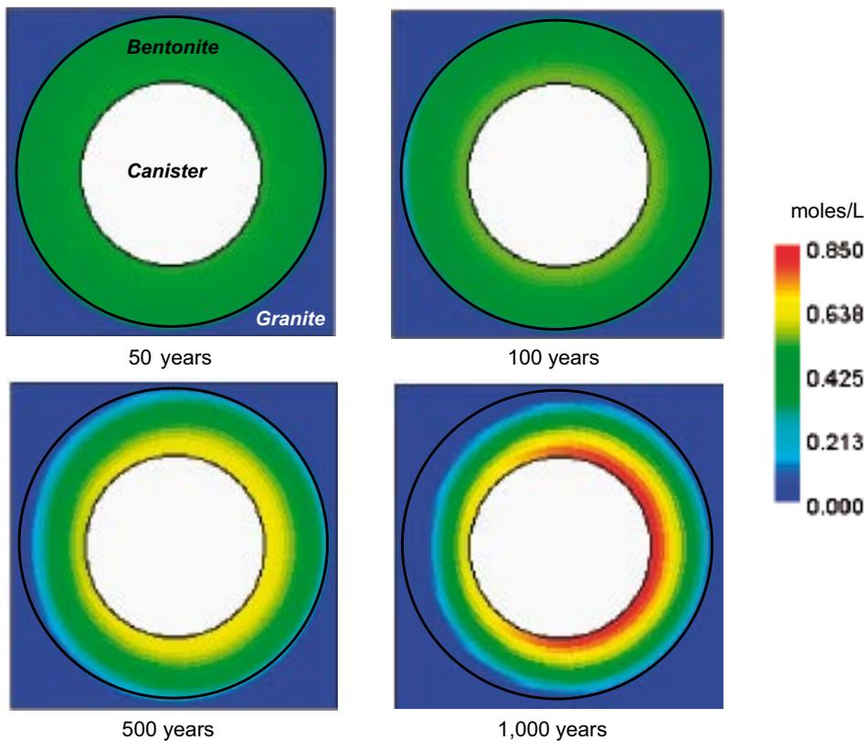
**Figure 5-76.** Predicted evolution of anhydrite content in the bentonite buffer during the thermal stage when Deponit CA-N is used as the bentonite buffer.
