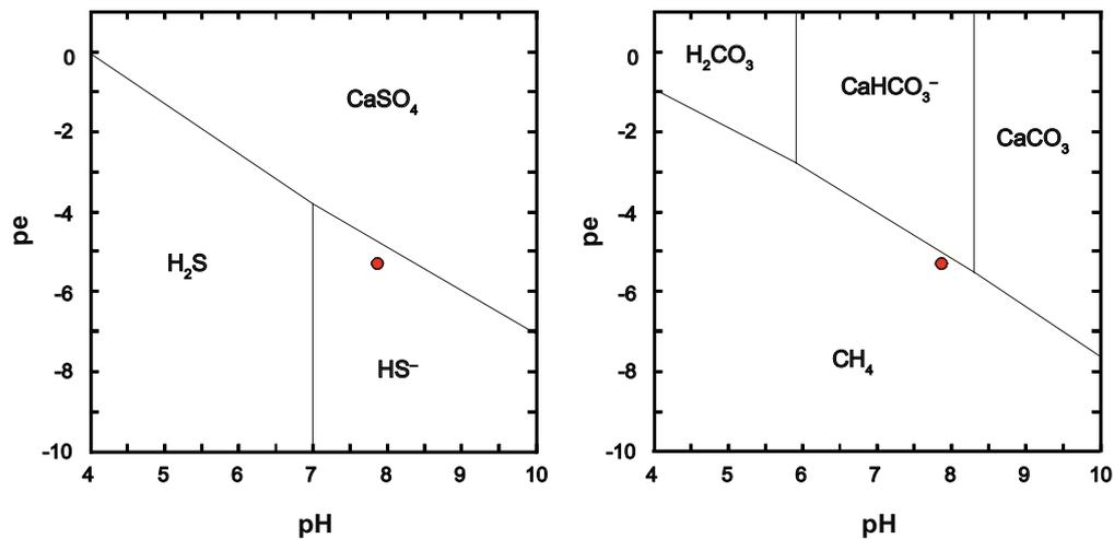
**Figure 5-17.** Sulphur and carbon predominance diagrams for the Laxemar high-salinity groundwater according to chemical composition from Table 2-1. The red dot represents the high-salinity groundwater from Laxemar.
