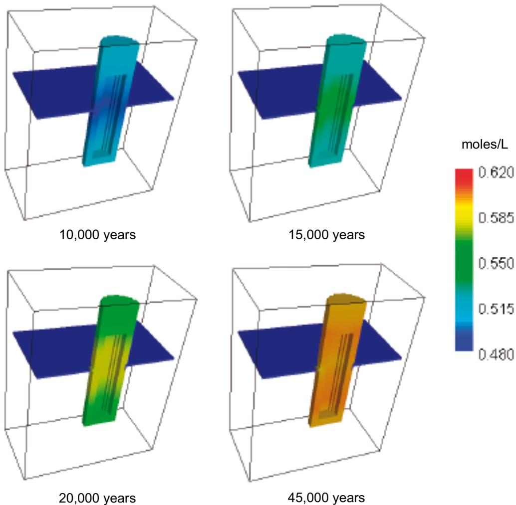
**Figure 5-31.** Predicted evolution of Ca occupancy in the exchanger of the bentonite. Note that before ice-melting water intrusion the Ca occupancy decreases, whereas after the intrusion the processes reverses and Ca occupancy increases.
