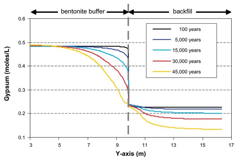
**Figure 5-46.** Evolution of gypsum concentration along the section 2 if Deponit CA-N bentonite is considered as buffer material. This mineral is always undersaturated in pore water and, consequently, it dissolves.
