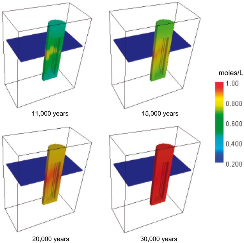
**Figure 5-21.** Predicted evolution of Ca occupancy in the cation exchanger of the bentonite after the intrusion of high-salinity water.
