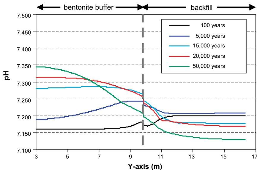
**Figure 5-49.** Graphic showing the predicted pH evolution as a function of time in section 2 (see Figure 5-34 for section location in the modelled domain).
