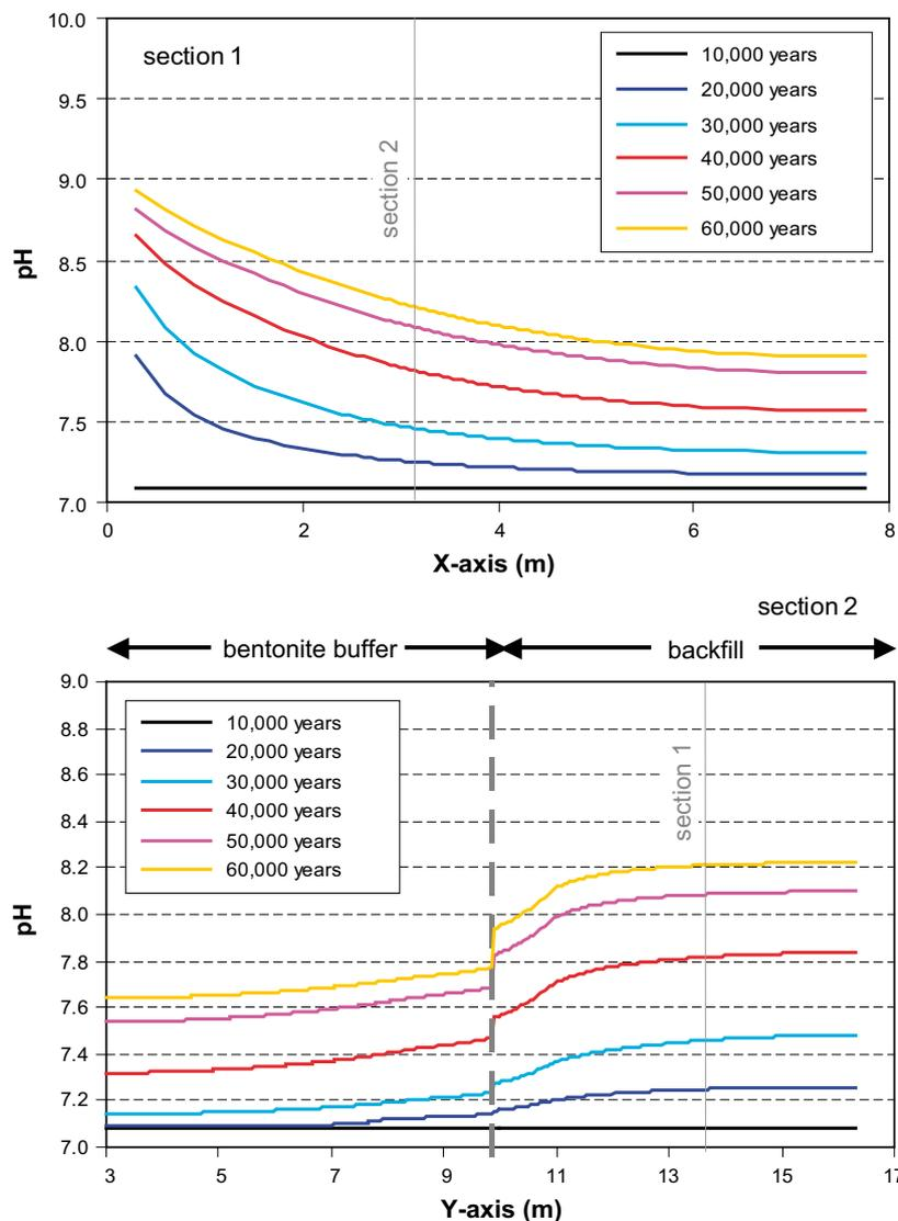
**Figure 5-50.** Graphics showing the predicted pH evolution after the ice-melting intrusion in two perpendicular sections (see location in Figure 5-34), one parallel to the deposition tunnel (upper graphic) and the other parallel to the deposition hole and including the backfill above it (lower diagram).
