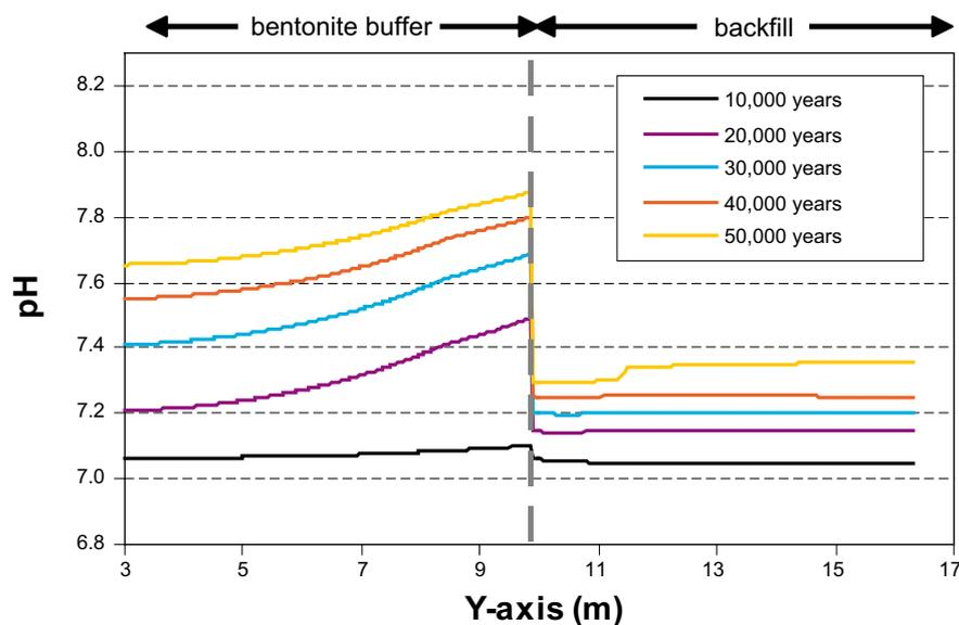
**Figure 5-47.** Evolution of pH along the section 2 after the intrusion of ice-melting waters. Deponit CA-N bentonite is considered as buffer material. The increase in pH is significantly higher than the observed when using MX-80 as a buffer material.
