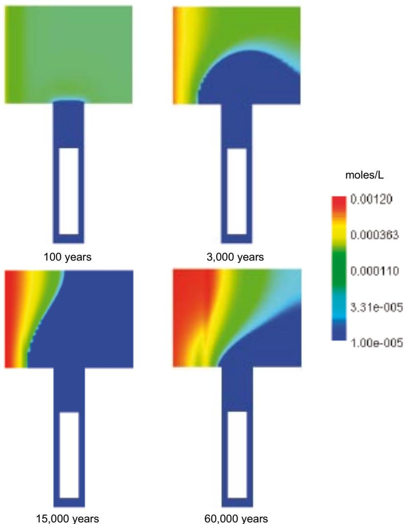
**Figure 5-36.** Predicted evolution of calcite in the modelled domain of the reference case with Friedland backfill and MX-80 bentonite buffer. Note that the scale bar is logarithmic.
