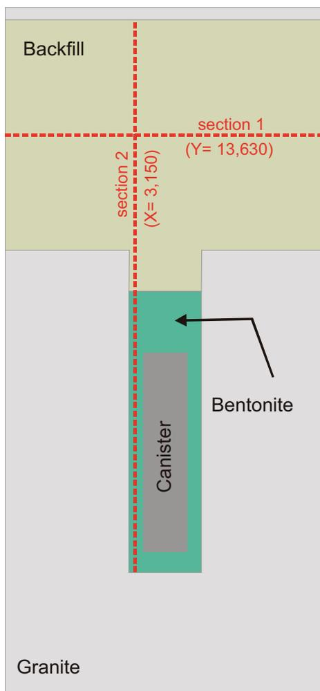
**Figure 5-34. Modelled domain of CASE-II, with selected sections, X and Y position in millimetres.**
