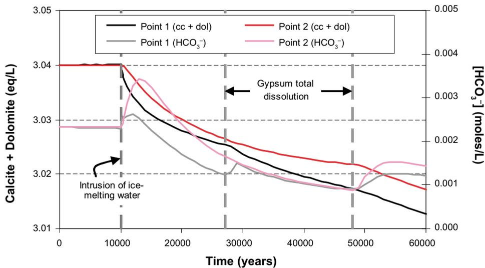
**Figure 5-28.** Predicted evolution of total carbonate concentration and carbonate minerals (calcite + dolomite) at two points in the bentonite as shown in Figure 5-10, (1) at the fracture level, and (2) far from the fracture intersection. Note that before ice-melting water intrusion the net amount of carbonates is maintained nearly constant, whereas after the intrusion it is strongly depleted and accompanied by an increase in aqueous carbonate concentration.
