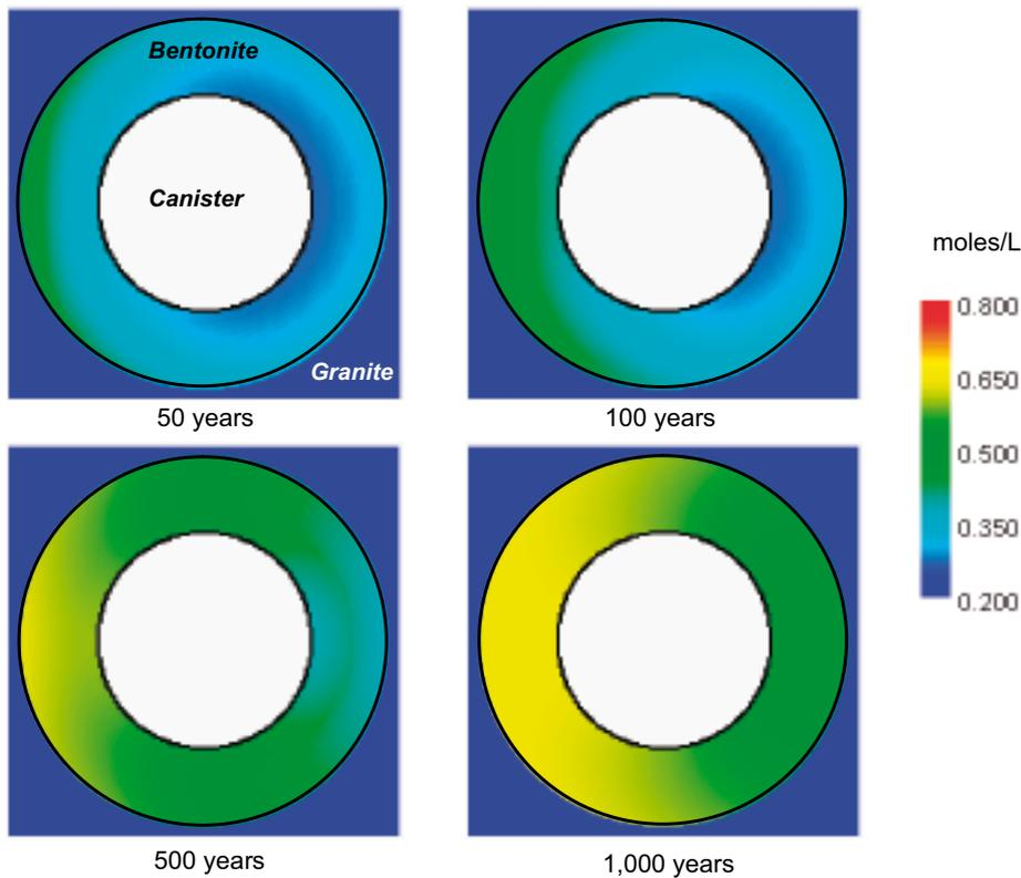
**Figure 5-70.** Evolution of  $[CaX_2]$  in the bentonite buffer during the thermal stage. The lower increase in the calcium occupancy in the right hand side of the buffer, especially during the initial 250 years, is due to the precipitation of anhydrite that fixes the calcium available in pore water.
