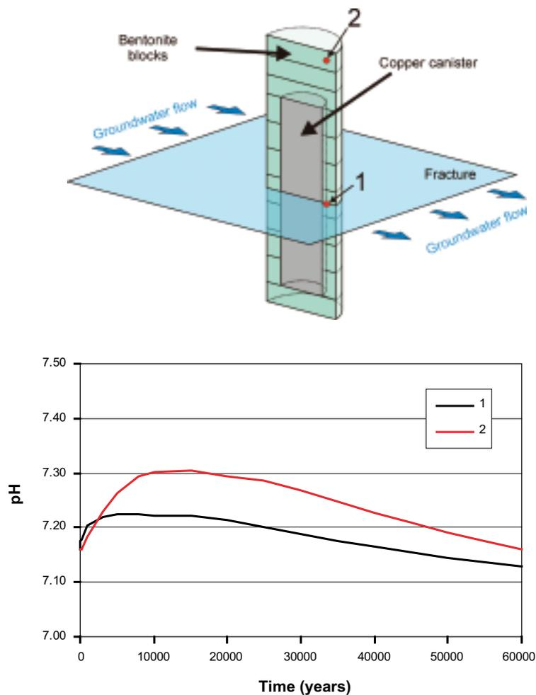
**Figure 5-10.** Evolution of pH through time for MX-80 bentonite with calcite and siderite (0.7 wt % each) at two bentonite points as shown in the upper graphic (1) close to the fracture, and (2) far from the fracture. pH pore water in bentonite increases with time reaching a maximum of 7.30 at point 2 and 7.22 at point 1 after 10,000 years of simulation. At the end of the simulation, after 60,000 years, pH values are similar to the initial ones.
