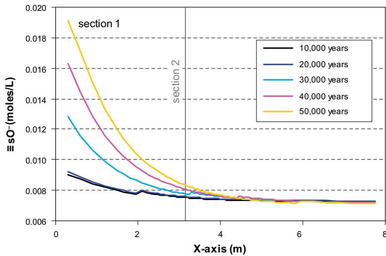
**Figure 5-40.** Predicted evolution of neutral (upper plot) and deprotonated (lower plot) surfaces of clay fraction in the backfill and bentonite buffer. Clay surfaces are progressively deprotonated as a response to the intrusion of high pH water.
