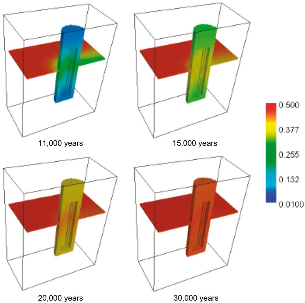
**Figure 5-19.** Evolution of aqueous calcium concentration through time in the modelled domain after the intrusion of high-salinity water at 10,000 years of simulation. Note the different scale with respect to Figure 5-4.
