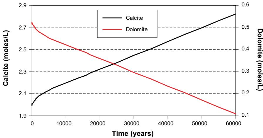
**Figure 5-24.** Predicted evolution of the dolomite and calcite content in the Deponit CA-N bentonite near the fracture zone (exact location as in Figure 5-7).
