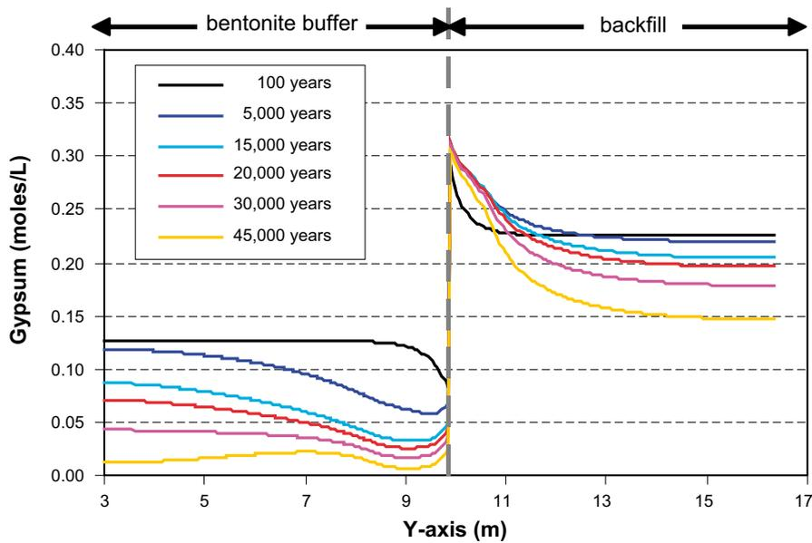
**Figure 5-37.** Evolution of gypsum along the section 2. Gypsum continuously dissolves in the whole domain except in the contact between the backfill and the buffer where it precipitates during the initial 5,000 years.
