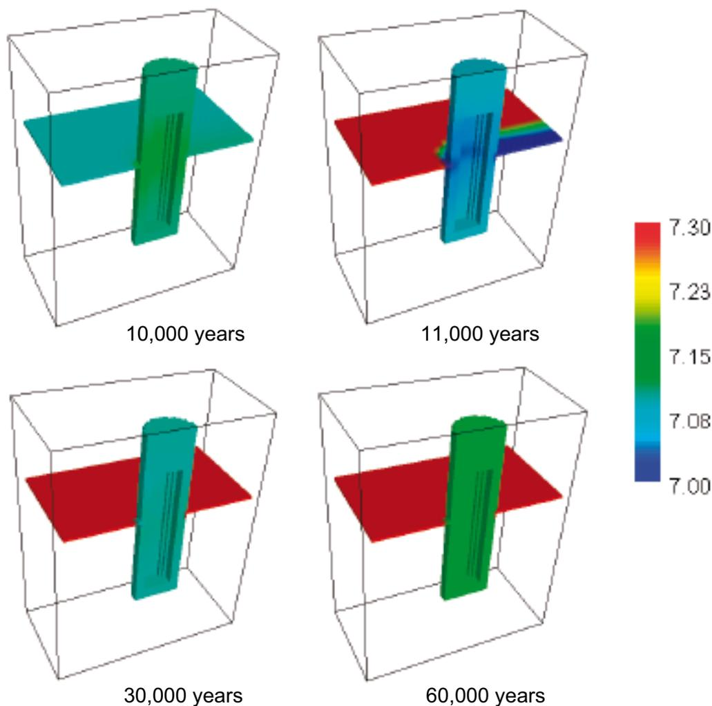
**Figure 5-32.** Predicted pH evolution of the system after the intrusion of high-salinity water at 10,000 years of simulation.
