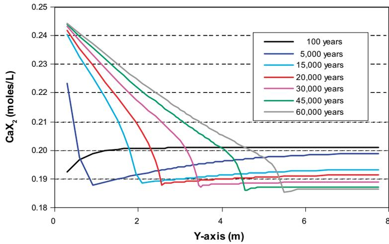
**Figure 5-58.** Graphic showing the predicted calcium occupancy in the exchanger of the bentonite in section 1 through the backfill. Note the reverse behaviour calcium once dolomite and gypsum have been dissolved, thus increasing the calcium occupancy in the exchanger.
