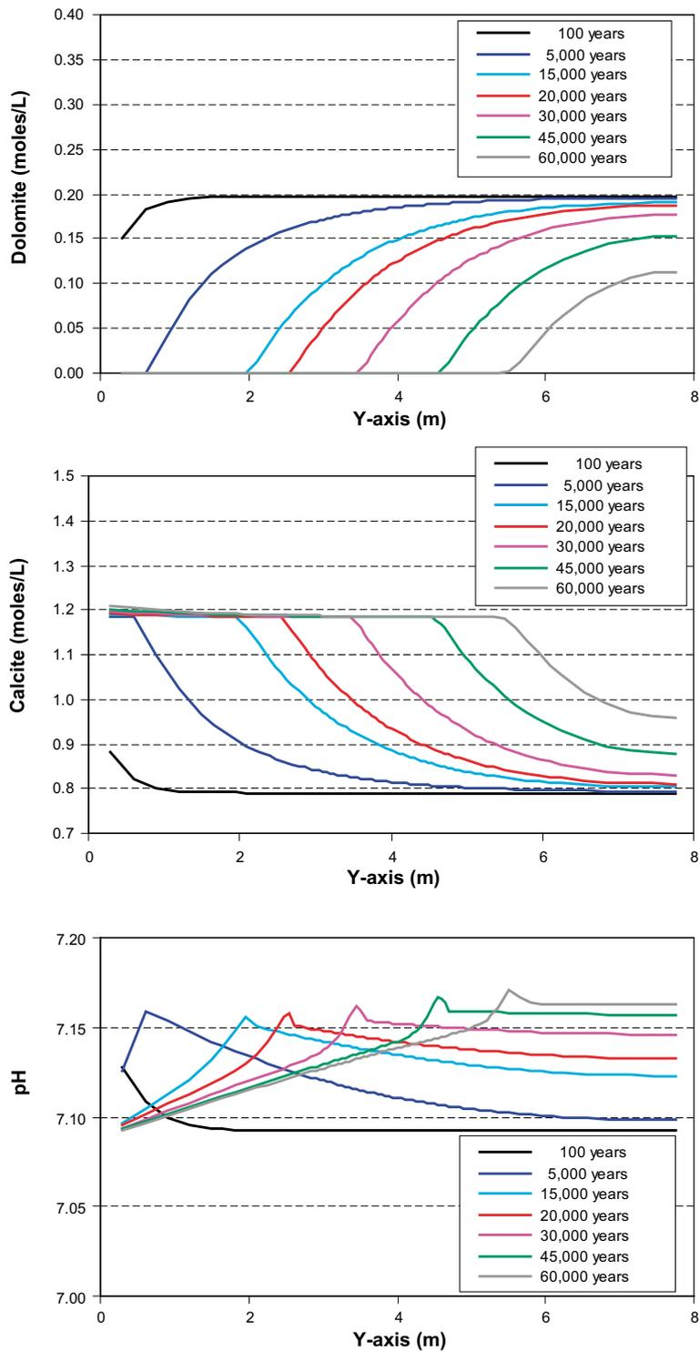
**Figure 5-57.** Graphics showing the predicted evolution of the amount of dolomite, calcite and pH in section 1, through the backfill.
