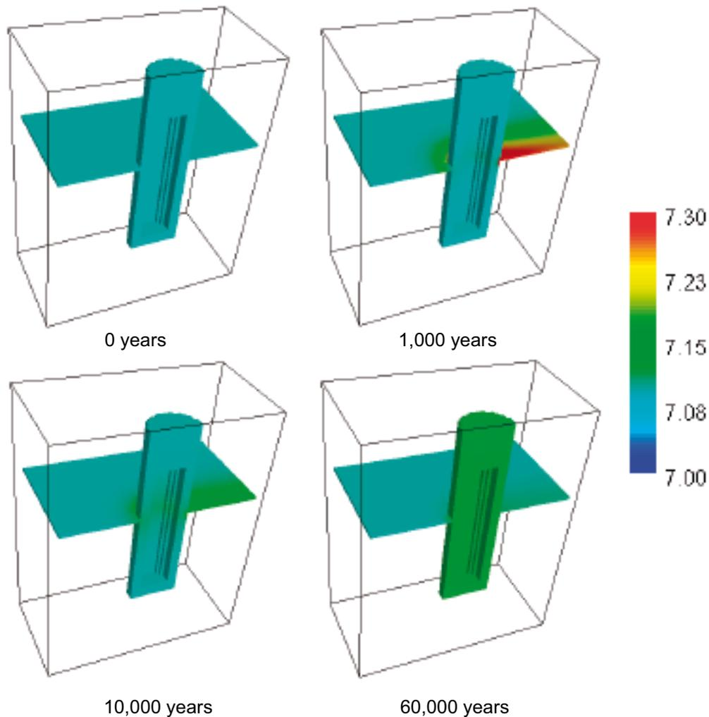
**Figure 5-3.** pH evolution in the simulated domain (MX-80 bentonite). Note the plume of slightly higher pH in the fracture plane caused by local calcite buffering, especially in the initial 1,000 years. As the pH in the bentonite zone increases, this plume becomes less evident. Maximum pH in the buffer is reached at the end of the simulation at values of 7.2.
