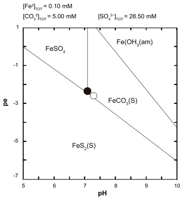
**Figure 5-9.** pH-pe diagram showing the Fe system and the initial pH and pe for bentonite pore water (black dot) and Forsmark groundwater (white dot). In both cases pH-pe conditions are close to pyrite and siderite equilibrium.
