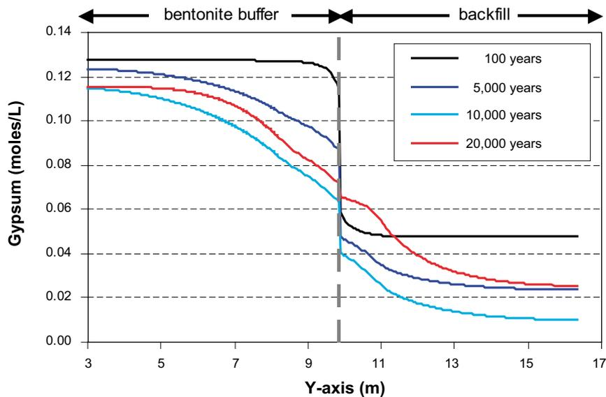
**Figure 5-55.** Predicted behaviour of gypsum in the system due to the intrusion of high-salinity groundwater. Note that after the high-salinity intrusion (10,000 years) gypsum precipitates again in both the backfill and the buffer.
