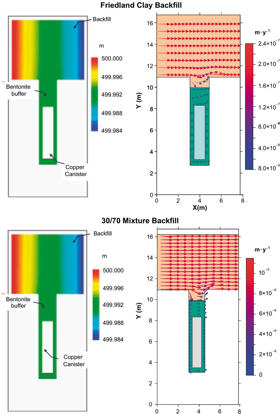
**Figure 5-35.** Hydraulic gradient and interstitial velocity field for CASE-II, considering the two types of backfill materials. Note that water flow velocities are much higher in the backfill than in the deposition hole.
