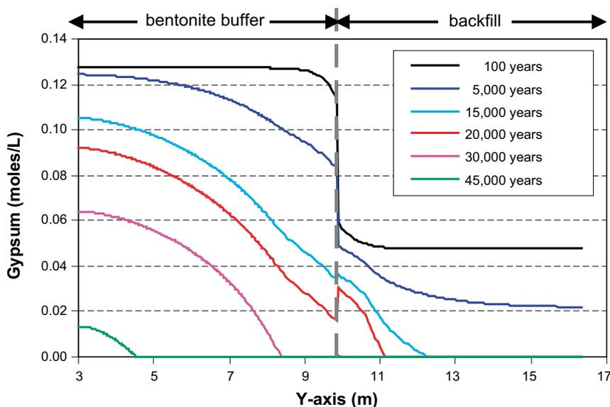
**Figure 5-48.** Graphic showing the predicted evolution of the gypsum content in both the backfill and the buffer in section 2 as a function of simulation time (see Figure 5-34 for section location).
