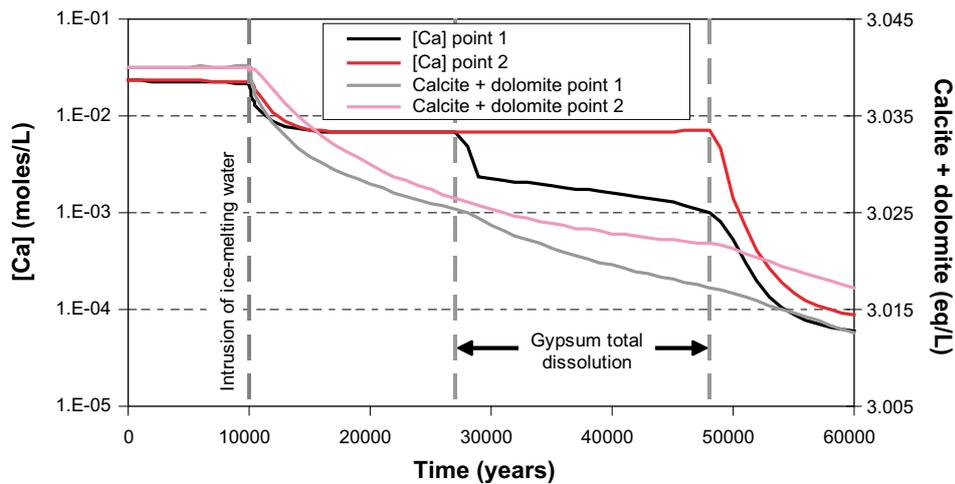
**Figure 5-27.** Predicted evolution of calcium concentration in pore water and carbonate minerals at two points in the bentonite as shown in Figure 5-10, (1) at the fracture level, and (2) far from the fracture intersection. The time at which ice-melting water intrudes into the system has been indicated. Gypsum total dissolution indicates the time range from total dissolution in those bentonite cells at the fracture level and total dissolution in the whole bentonite.
