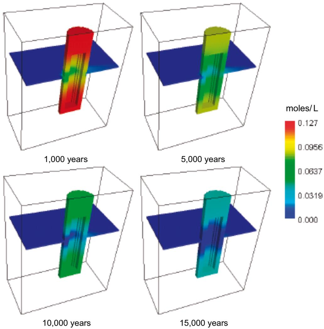
**Figure 5-5.** Dissolution of gypsum during the simulation period. It is interesting to observe the fast dissolution at the fracture-bentonite interface: at 1,000 years gypsum concentration is a half of the initial inventory, and at 20,000 years it has almost been dissolved in the whole domain.
