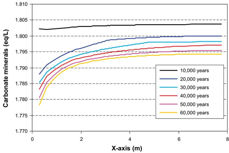
**Figure 5-60.** Predicted evolution of the net amount of carbonate minerals in the backfill in section 1.
