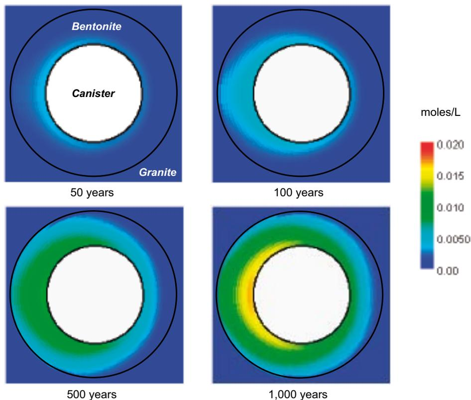
**Figure 5-68.** Evolution of dolomite concentration in the buffer section at fracture level. Note the progressive precipitation of this mineral through time. The smaller precipitation of dolomite in the right hand side part of the bentonite domain, especially during the initial times, is caused by the opposite behaviour of anhydrite, which dissolves in the left hand side part and precipitates in the right hand side part (see Figure 5-69).
