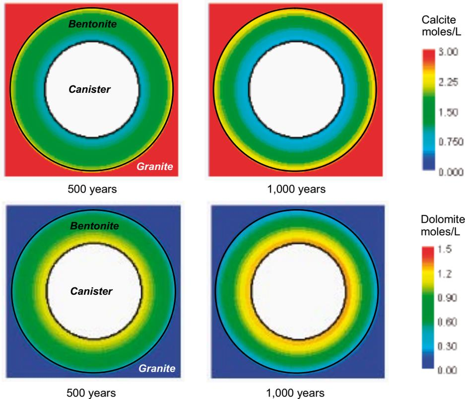
**Figure 5-77.** Predicted evolution of calcite (upper graphics) and dolomite (lower graphics) in the bentonite buffer during the thermal stage when Deponit CA-N is used as the bentonite buffer. Note that dolomite replaces calcite close to the canister and the reverse occurs in the cooler part of the system, near the granite-bentonite boundary.
