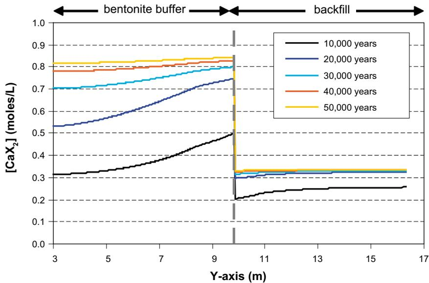
**Figure 5-43.** Predicted calcium occupancy in the exchanger of the bentonite due to the intrusion of high-salinity groundwater in the section 2. The increase in the  $CaX_2$  concentration in the exchanger is a consequence of the Ca-rich nature of the high-salinity groundwater.
