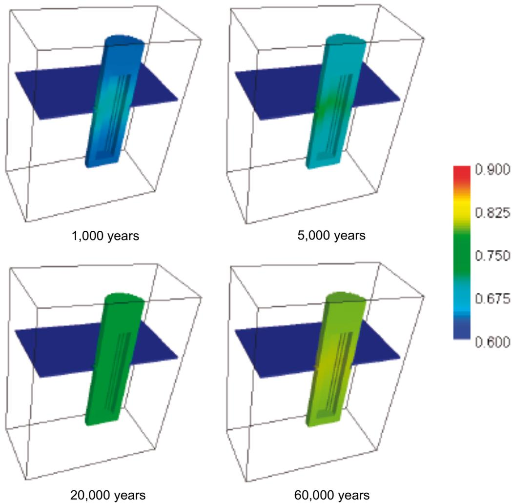
**Figure 5-25.** Predicted evolution of Na occupancy in the cation exchanger of the bentonite.
