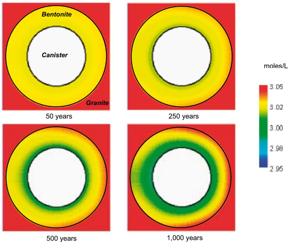
Figure 5-71. Predicted evolution of quartz content in the bentonite buffer during the thermal stage.
