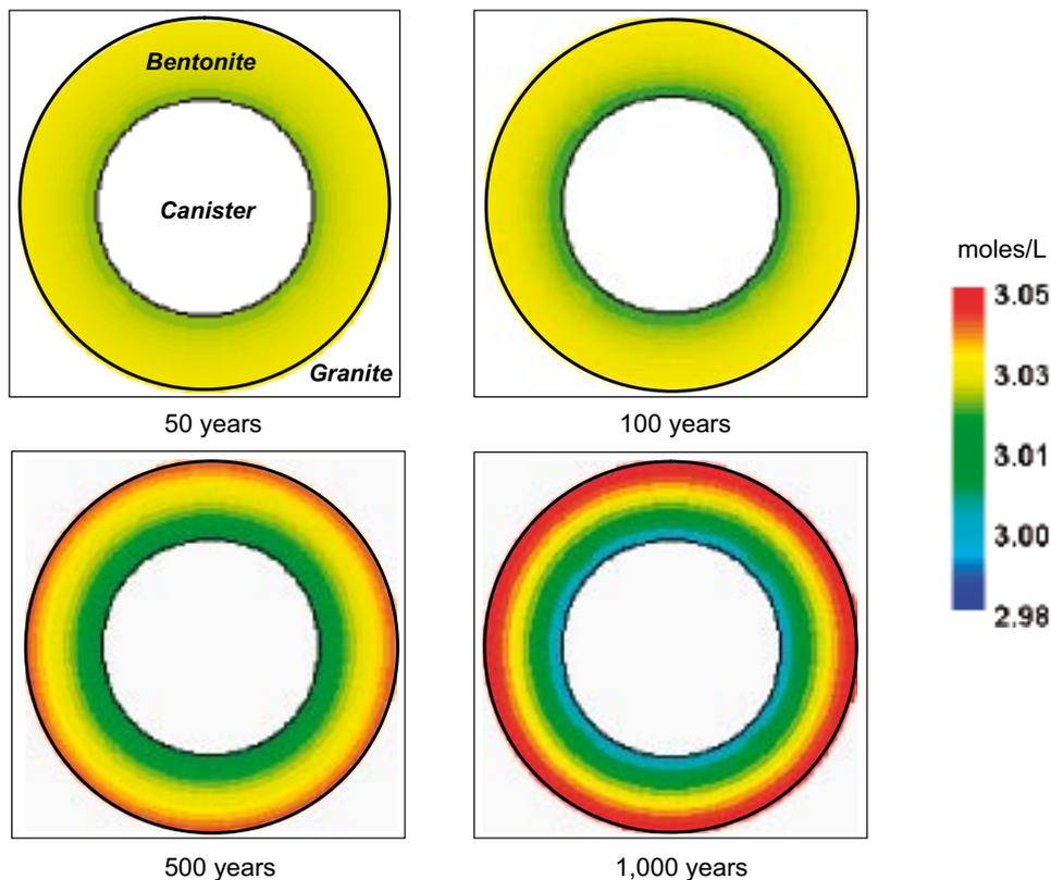
**Figure 5-74.** Evolution of quartz concentration in the bentonite buffer. It is clearly observable the mobilization of silica from warmer zones to cooler zones through time. Quartz progressively dissolves in the areas closer to canister and re-precipitates in the outer rims of the bentonite sections. Solute transport and reaction from granite to bentonite is not allowed in the simulations.
