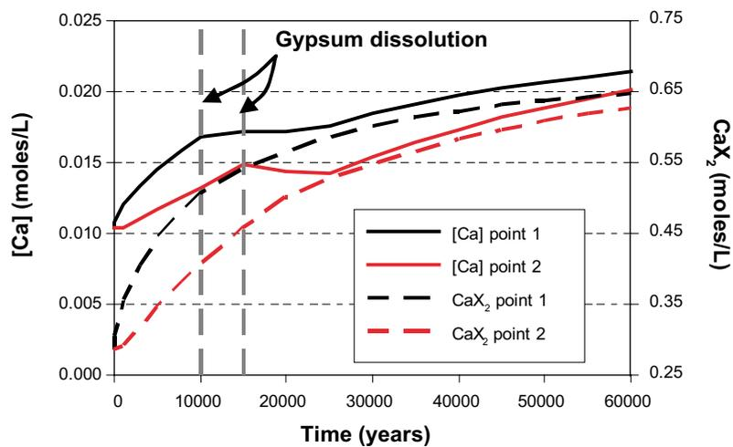
**Figure 5-13.** Predicted evolution of calcium concentration in pore water and Ca occupancy in the exchanger at two points in the bentonite as shown in Figure 5-10, (1) at the fracture level, and (2) far from the fracture intersection. Gypsum complete dissolution in the two points is shown for comparison. Note that the concentration of calcium is always lower in point 2 respect to point 1, and consequently the Ca occupancy in the exchanger is also lower.
