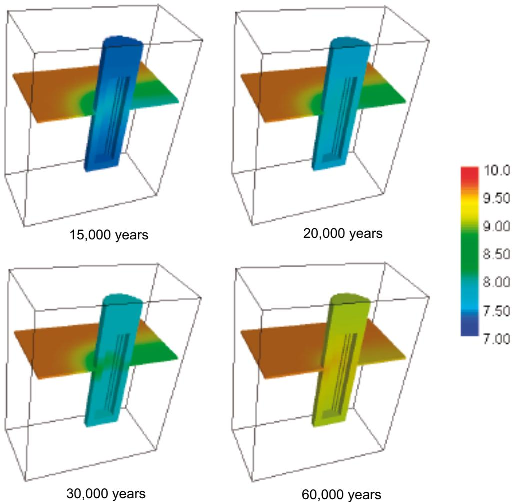
**Figure 5-26.** Predicted pH evolution of the system after the intrusion of ice-melting water at 10,000 years of simulation.
