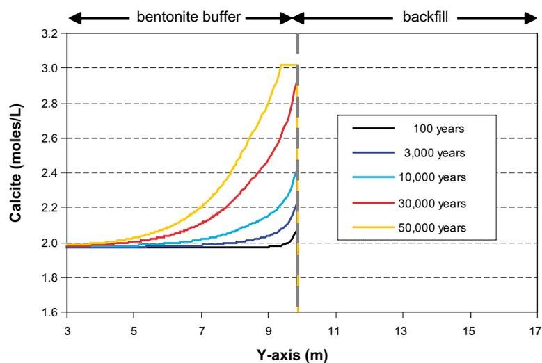
**Figure 5-45.** Evolution of dolomite (upper plot) and calcite (lower plot) concentrations along the section 2 if Deponit CA-N bentonite is considered as buffer material. Because of this mineral evolution, pH undergoes a slight increase.
