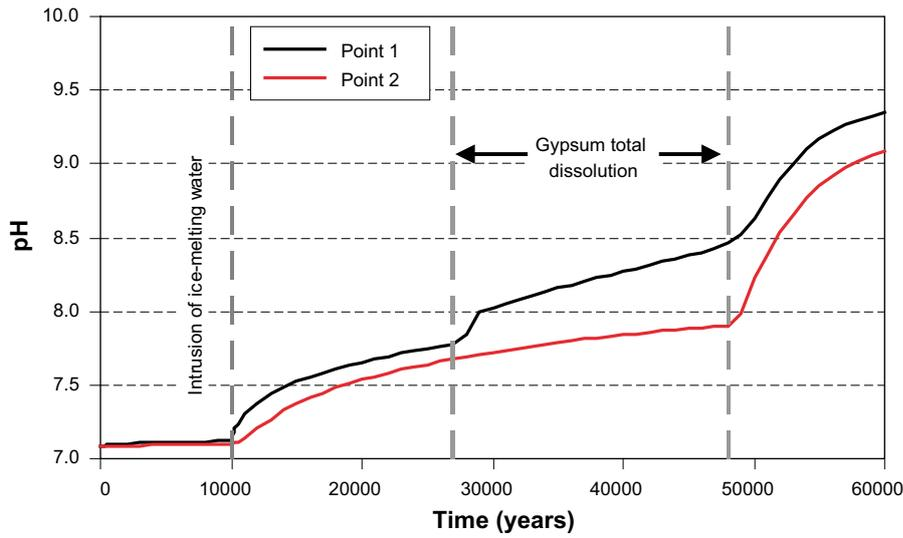
**Figure 5-29.** Graphic showing the detailed evolution of pH at two points in the bentonite as shown in Figure 5-10, (1) at the fracture level, and (2) far from the fracture intersection. Note the three jumps in pH related to the intrusion of ice-melting water and gypsum dissolution.
