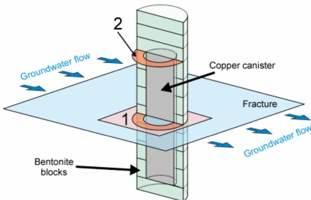
**Figure 5-65.** Location of the two sections considered in CASE-III. Section 1 corresponds to the fracture level and granitic groundwater effect is expected, whereas section 2 is far from the fracture level, and therefore geochemical changes are only expected as a consequence of the thermal gradient.
