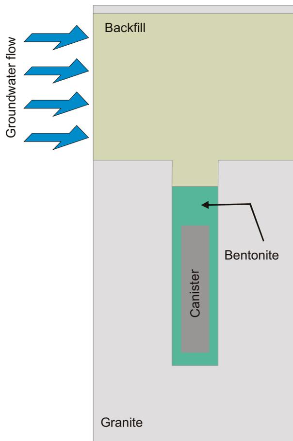
*Figure 5-1. Modelled domain in the CASE-II.*
