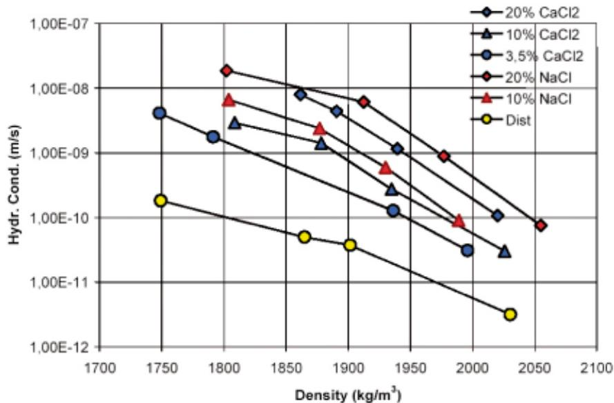
**Figure 3-3.** Hydraulic conductivity vs. clay density in experiments where water with variable salinity is percolated. From /Pusch et al. 2003/.
