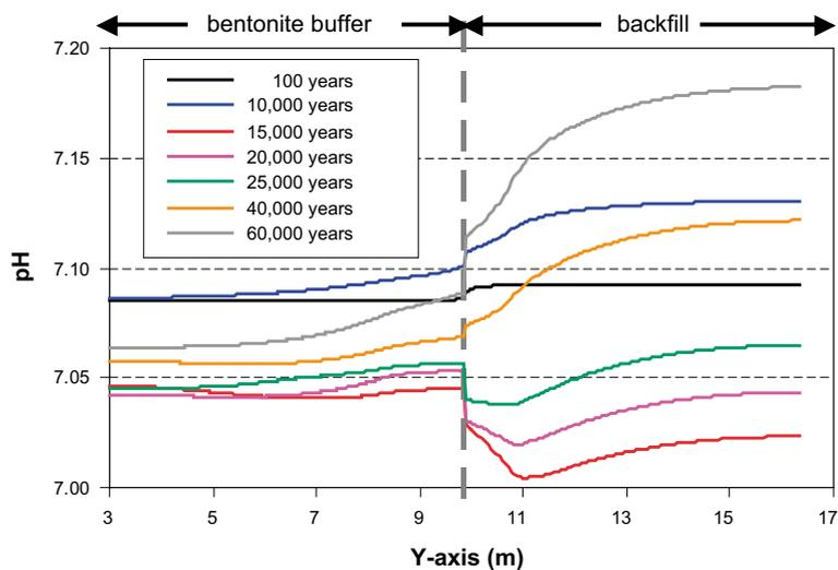
**Figure 5-62.** Predicted evolution of pH in the backfill and the buffer during high-salinity groundwater intrusion in section 2.
