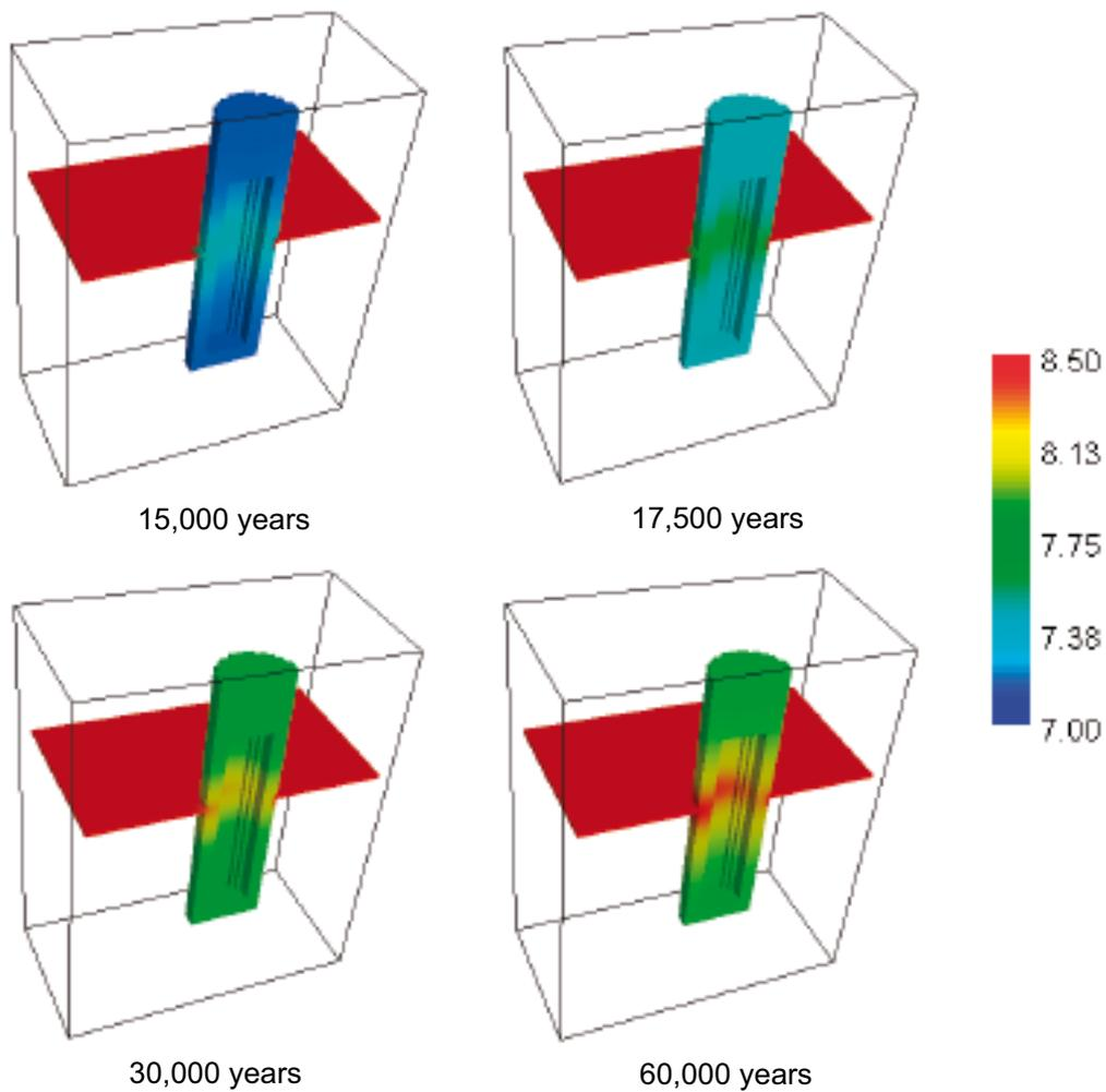
**Figure 5-14.** Predicted pH evolution of the system after the intrusion of ice-melting water at 10,000 years of simulation.
