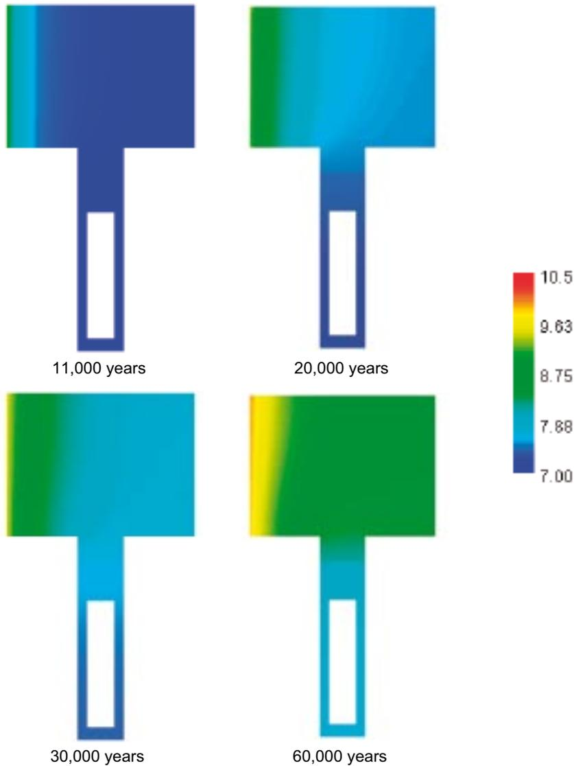
**Figure 5-59.** Predicted pH evolution after the intrusion of ice-melting water, which interacts with the backfill and the buffer.
