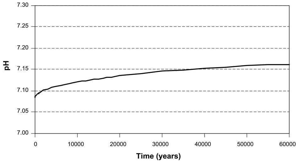
**Figure 5-23.** Predicted pH evolution in the Deponit CA-N bentonite pore water near the fracture zone (exact location as in Figure 5-7).
