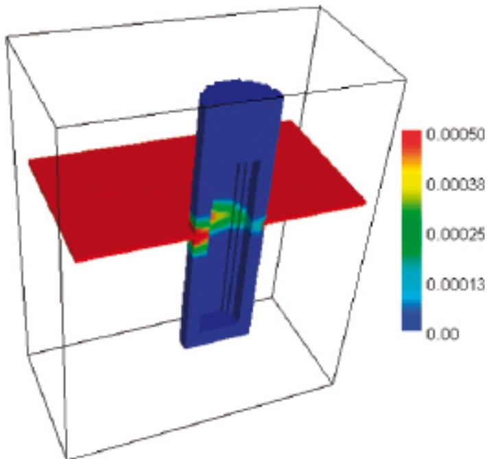
**Figure 5-8.** Precipitation of secondary calcite at the end of the simulation (60,000 years). This precipitation is responsible for the decrease of pH observed in the latest stages. Calcite concentration in the fracture plane is much higher than indicated in the scale bar (11.5 mol/L). The scale bar (mol/L) has been limited to a very narrow range for a better observation in the bentonite.
