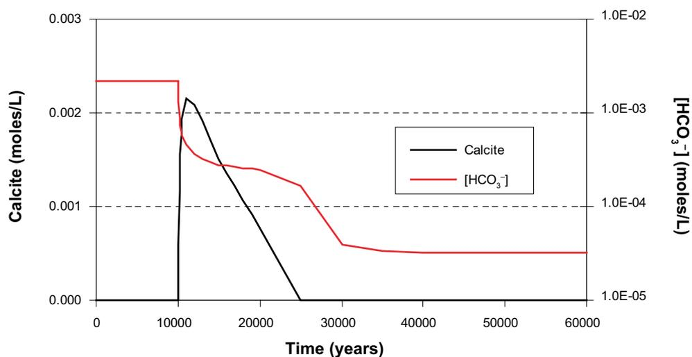
**Figure 5-20.** Predicted evolution of the aqueous carbonate concentration and calcite content in the bentonite near the fracture zone (exact location as in Figure 5-7) due to the intrusion of a high-salinity groundwater after 10,000 years of simulation.
