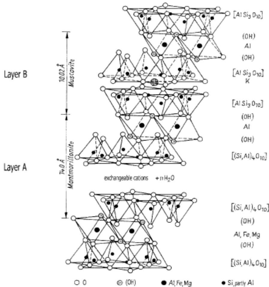
**Figure 3-2.** Structure of the Friedland Clay, alternating muscovite and montmorillonite layers. From /Pusch et al. 2003/.
