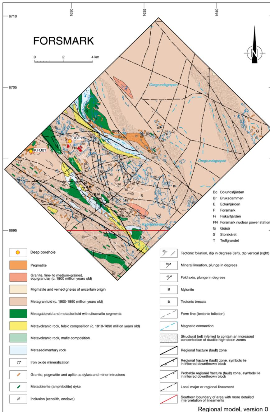
**Figure 2-1.** 2D cartographic model for the bedrock geology at the surface, both onshore and offshore in Forsmark area. After /SKB 2002/.
