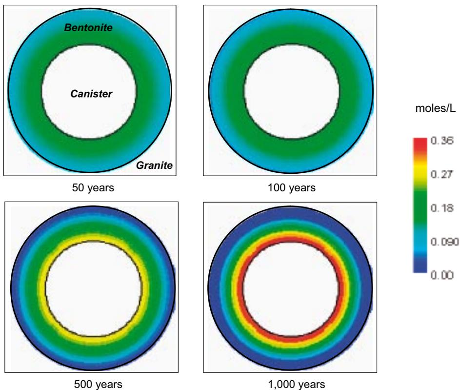
**Figure 5-73.** Predicted evolution of anhydrite content in the bentonite buffer during the thermal stage in a section located away from a hydraulically conductive fracture. Note the symmetric changes in the modelled domain. Diffusive transport of calcium and sulphate leads to dissolution of anhydrite in the outer (cooler) parts of the section and subsequent re-precipitation in the inner (warmer) zones. Compare the different evolution with Figure 5-69.
