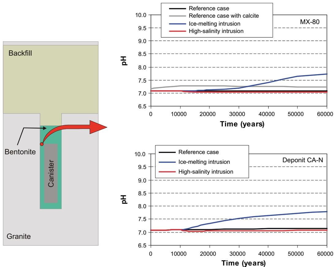
**Figure 5-63.** Predicted pH evolution in the bentonite buffer close to the upper part of the canister.
