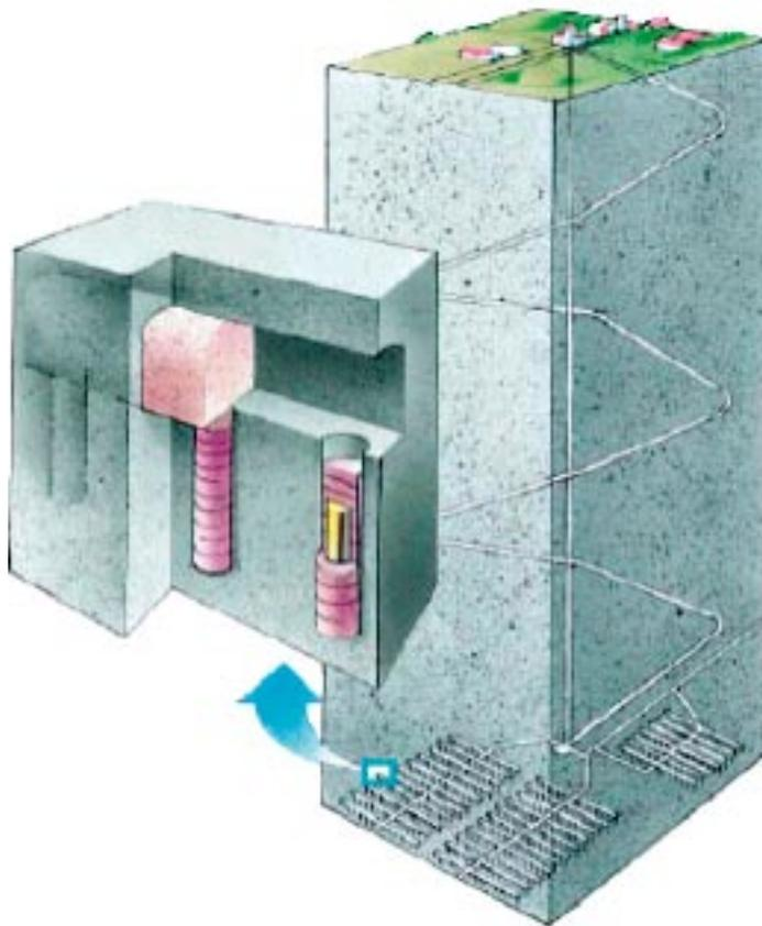
**Figure 3-1.** KBS-3 concept for storage of HLNW designed by SKB. Spent nuclear fuel will be stored in copper canisters buried at depth and surrounded by compacted bentonite blocks.
