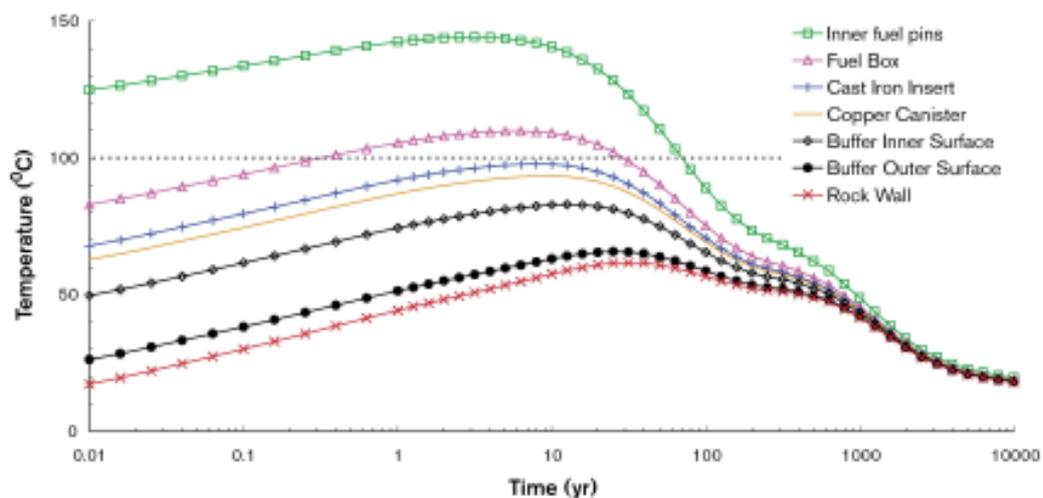
**Figure 5-64.** Calculated thermal evolution of the near field. Note that temperatures in the buffer reach up to 80°C in the initial times of spent fuel storage. Adapted from /SKB 2004b/.
