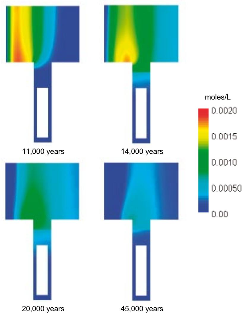
**Figure 5-53.** Predicted precipitation and dissolution of calcite during the intrusion of high-salinity groundwater into the system.
