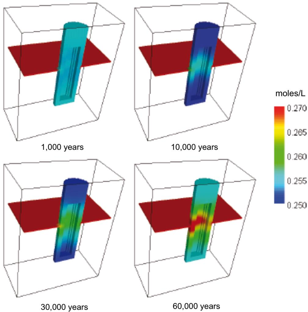
**Figure 5-12.** Evolution of calcite content for MX-80 bentonite with calcite and siderite (0.7 wt % each). Note the dissolution of calcite during the first 10,000 years of simulation and its precipitation thereafter until the end of the simulation.
