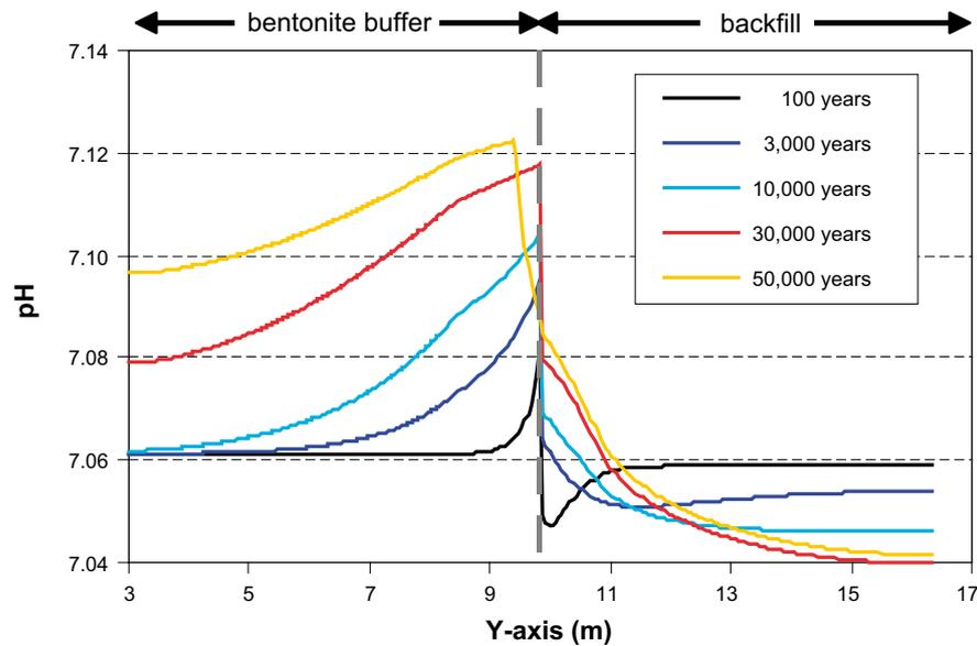
**Figure 5-44.** Evolution of pH along the section 2 if Deponit CA-N bentonite is considered as buffer material. The increase in pH in the bentonite buffer close to the backfill is related to dolomite dissolution.
