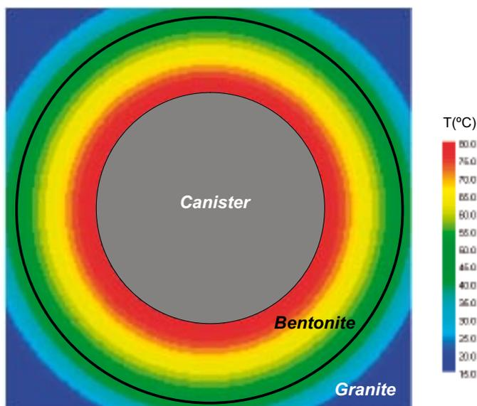
**Figure 5-66.** Modelled section in the CASE-III showing the temperature field considered in the model. Scale bar indicates the temperature range in °C.
