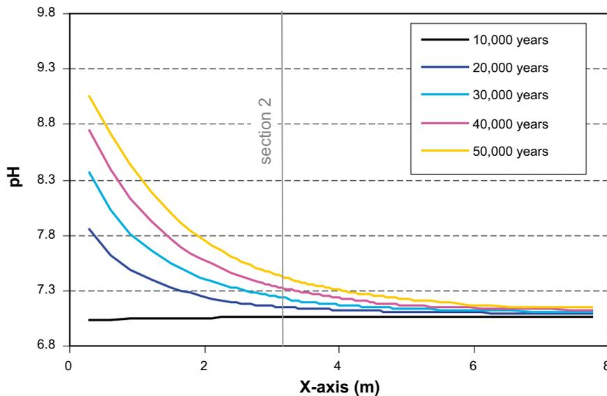
**Figure 5-39.** Plot showing the predicted pH evolution after the ice-melting intrusion in section 1 (transect through the backfill,  $X=3.15$  m). pH increases through time due to the alkaline character of the inflow groundwater after 10,000 years.
