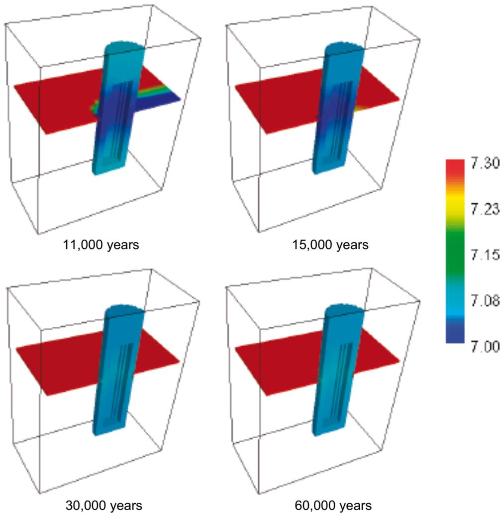
**Figure 5-18.** Predicted pH evolution of the system after the intrusion of high-salinity water at 10,000 years of simulation.
