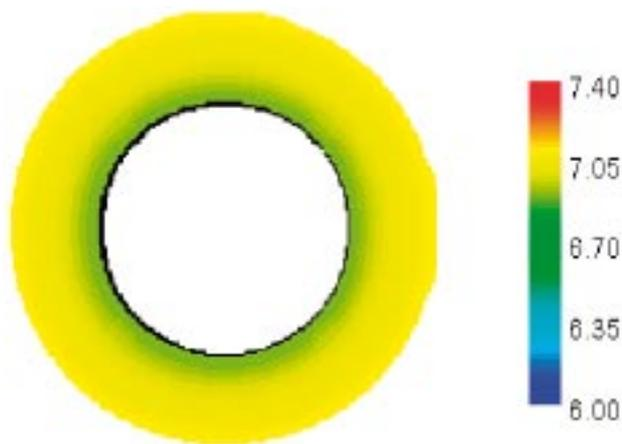
**Figure 5-72.** pH of MX-80 bentonite pore water after 1,000 years simulation. Note the small variation in pH, especially when compared with Figure 5-67.
