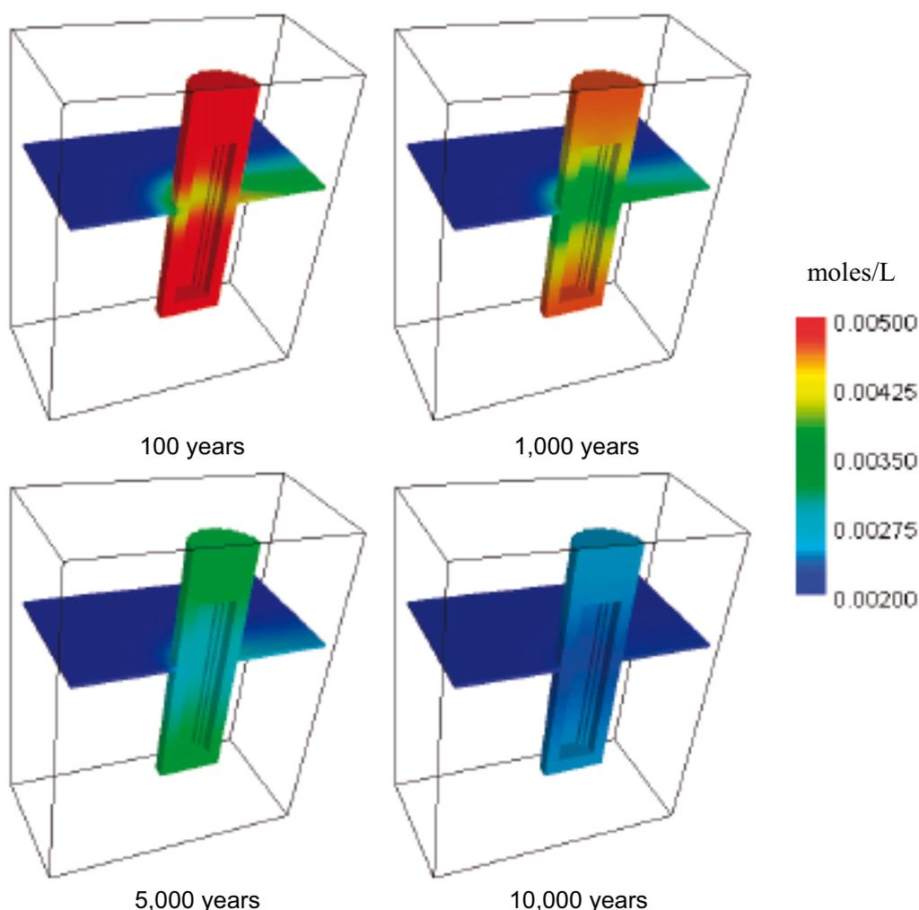
**Figure 5-11.** Predicted time and spatial evolution of aqueous carbonate in the system. Note that aqueous carbonate diffuses out from bentonite until the same concentration as in Forsmark groundwater is reached after 10,000 years of simulation.
