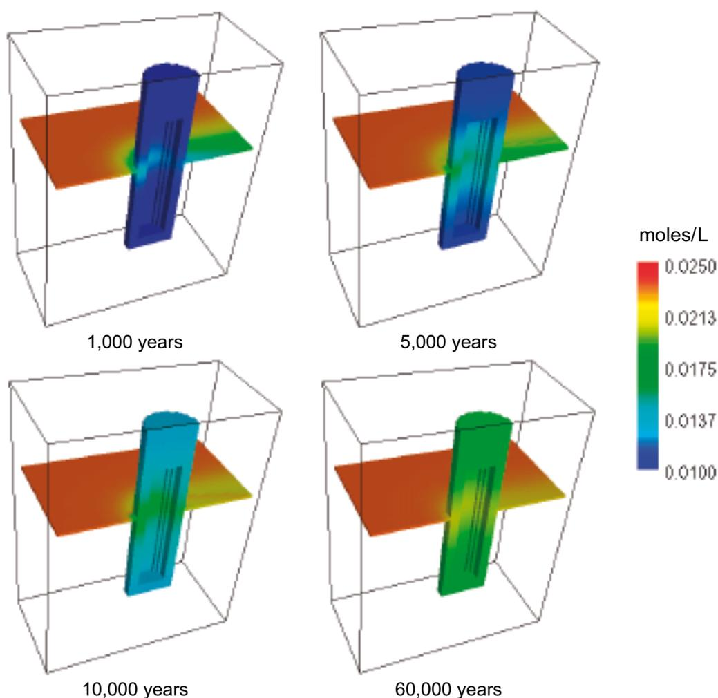
**Figure 5-4.** Evolution of aqueous calcium concentration through time in the modelled domain. Calcium concentration in pore water increases in MX-80 bentonite buffer whereas in the fracture a plume of lower calcium concentration is observed.
