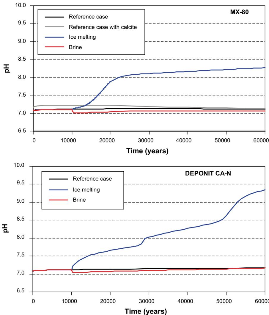
**Figure 5-33.** Comparison of predicted pH evolution for the different scenarios considered in CASE-I at a point in the bentonite close to the fracture in granite, as shown in Figure 5-7.
