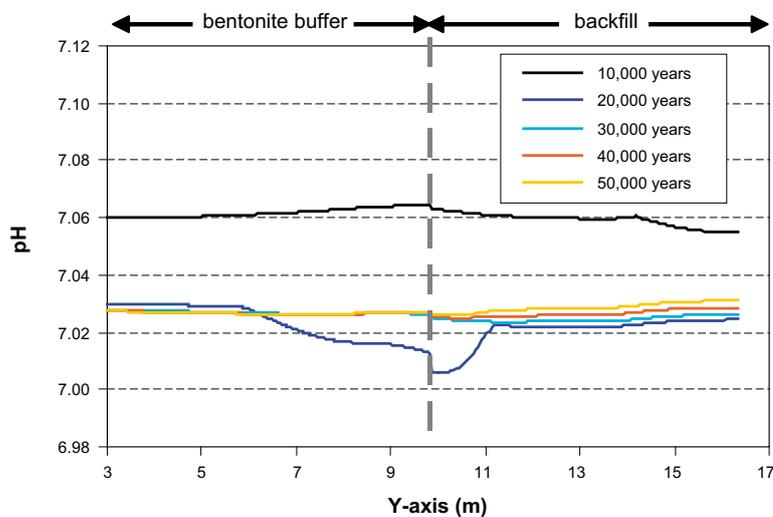
**Figure 5-41.** Plot showing the predicted evolution of pH after the intrusion of high-salinity groundwater after 10,000 years of simulation in section 2.
