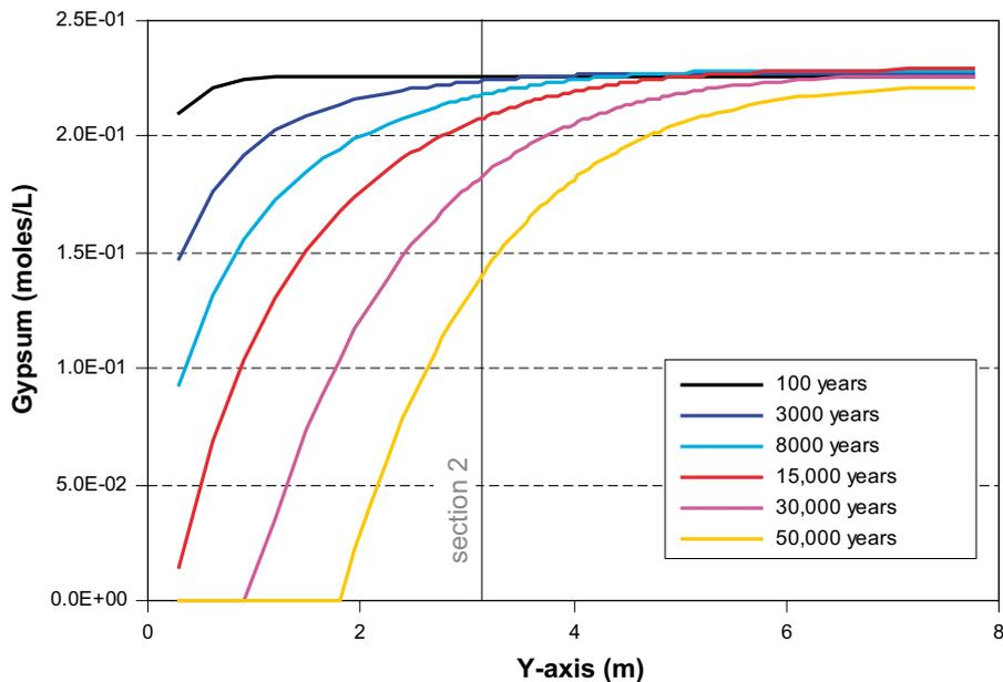
**Figure 5-38.** Evolution of gypsum along the section 1 (backfill transect). Gypsum dissolution in the backfill is enhanced by the inflow of the Forsmark groundwater.
