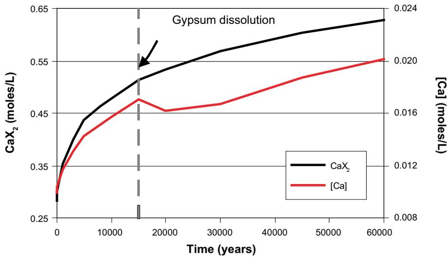
**Figure 5-7.** Predicted evolution of calcium occupancy in the exchanger and calcium concentration of bentonite pore water in the bentonite close to the fracture as shown in upper graphic. The time at which gypsum is totally dissolved is also shown.
