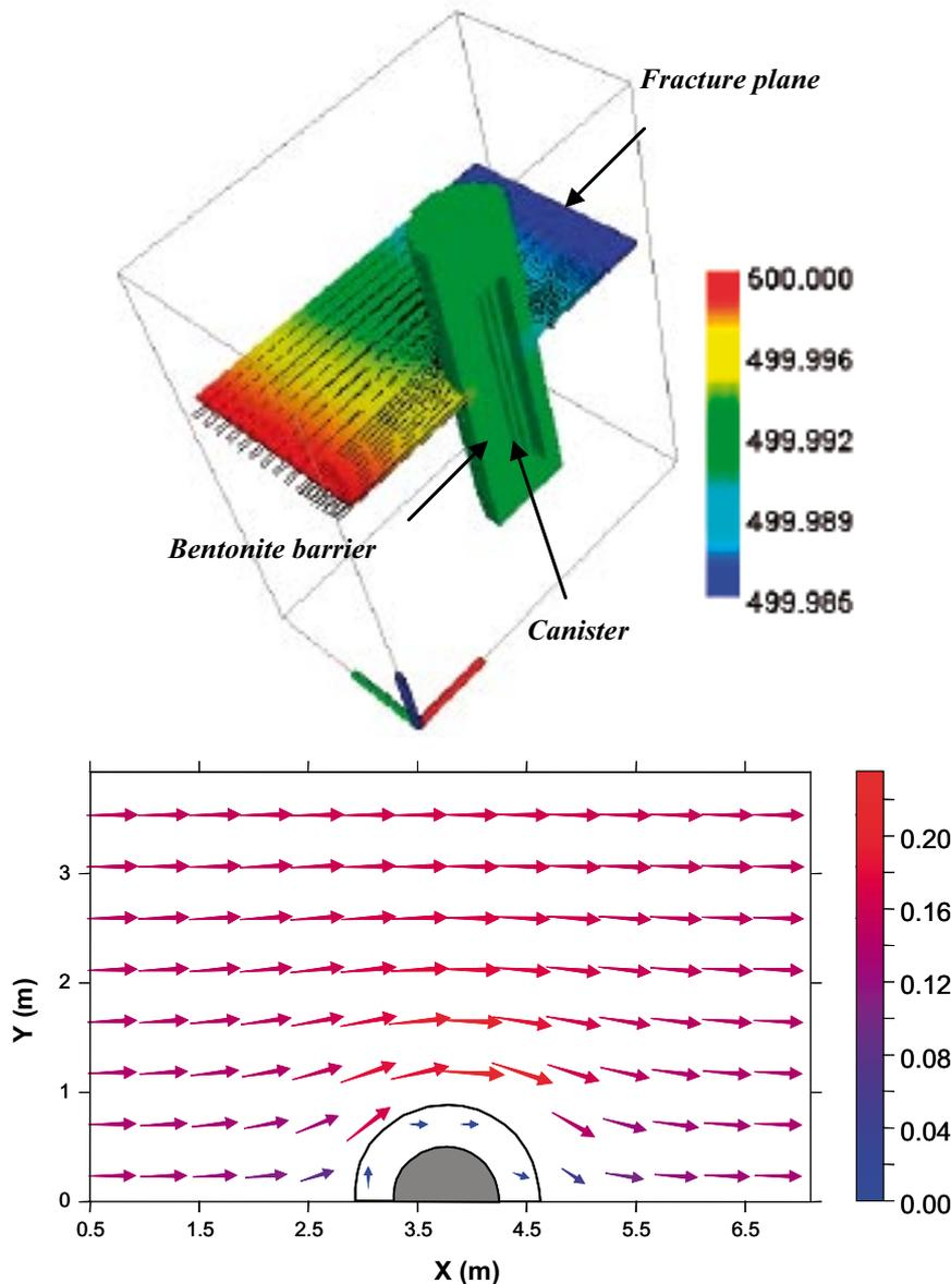
**Figure 5-2.** (top) Fluid head (in colour) and flow vectors of the CASE-I model. Water flows from the left boundary to the right and flow vectors are diverted close to the bentonite barrier. Scale bar in metres. (bottom). Water flow velocities (in m·yr<sup>-1</sup>) in the fracture plane. Velocities are much lower (close to 0) in the bentonite (grey area).
