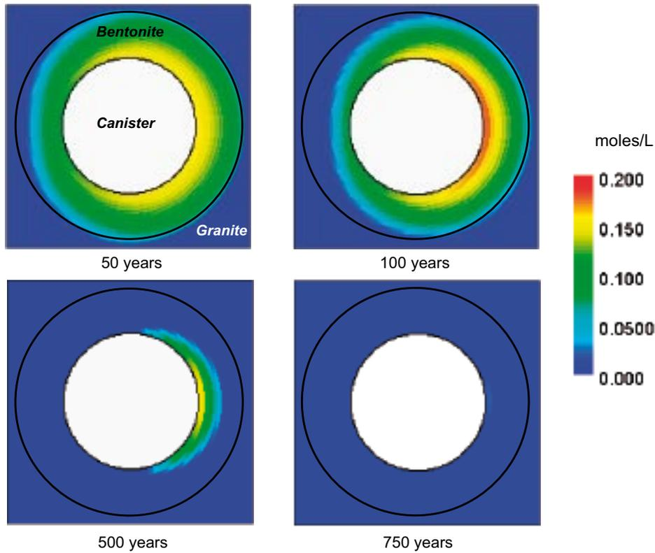
**Figure 5-69.** Predicted evolution of anhydrite content in the bentonite buffer during the thermal stage. Note the coeval dissolution and precipitation of this mineral in different parts of the bentonite in the first 100 years. Afterwards, anhydrite dissolves to disappear in less than 800 years.
