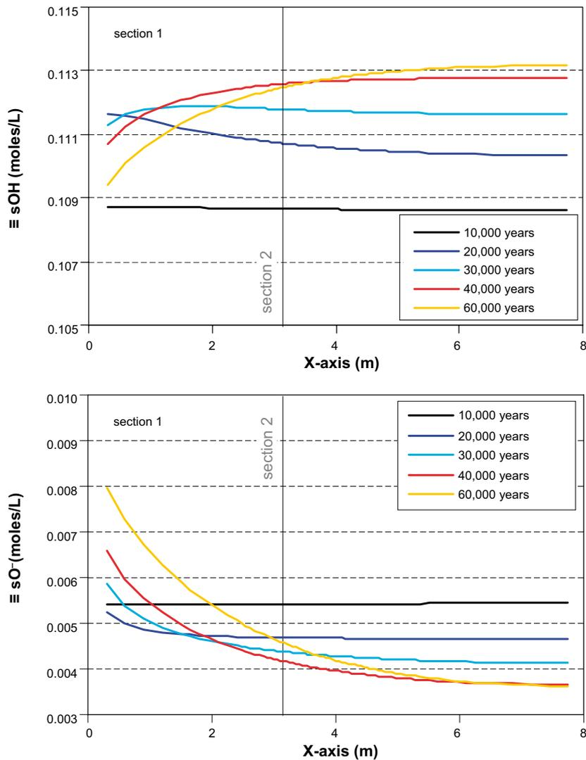
**Figure 5-51.** Graphics showing the predicted evolution of neutral (upper graphic) and deprotonated (lower graphic) surfaces of clay fraction in the backfill.
