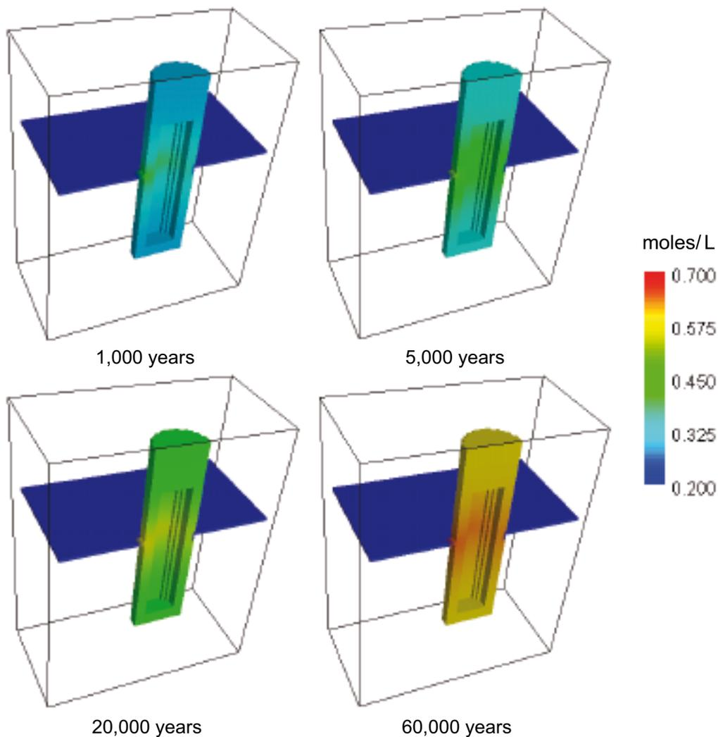
**Figure 5-6.** Predicted evolution of Ca occupancy in the cation exchanger of the bentonite.
