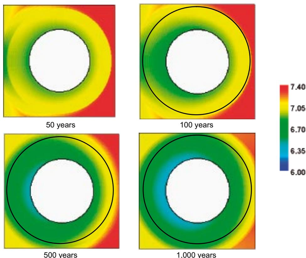
**Figure 5-67.** Predicted pH evolution of the system during the thermal stage at the fracture level where MX-80 is used as a bentonite buffer.
