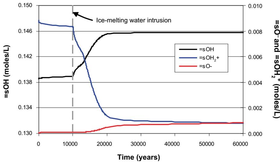
Figure 5-15. Predicted evolution of the surface acidity (Z sites in Table 5-3) of the clay fraction in the bentonite at point 1 as indicated in Figure 5-10.
