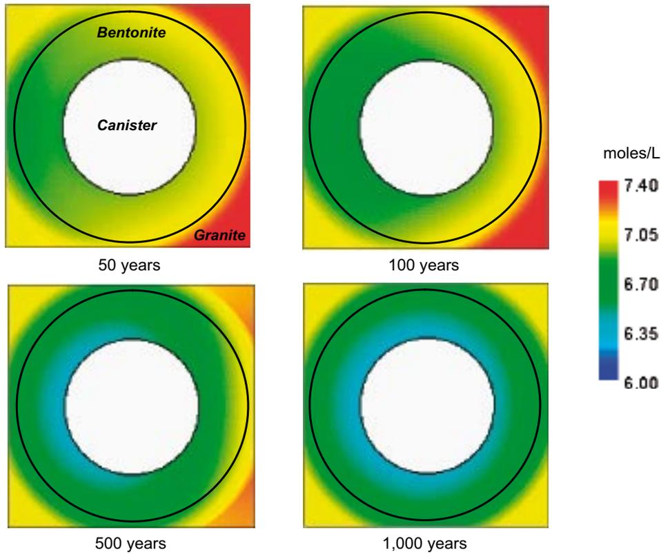
**Figure 5-75.** Predicted pH evolution of the system during the thermal stage. Deponit CA-N is used as a bentonite buffer.
