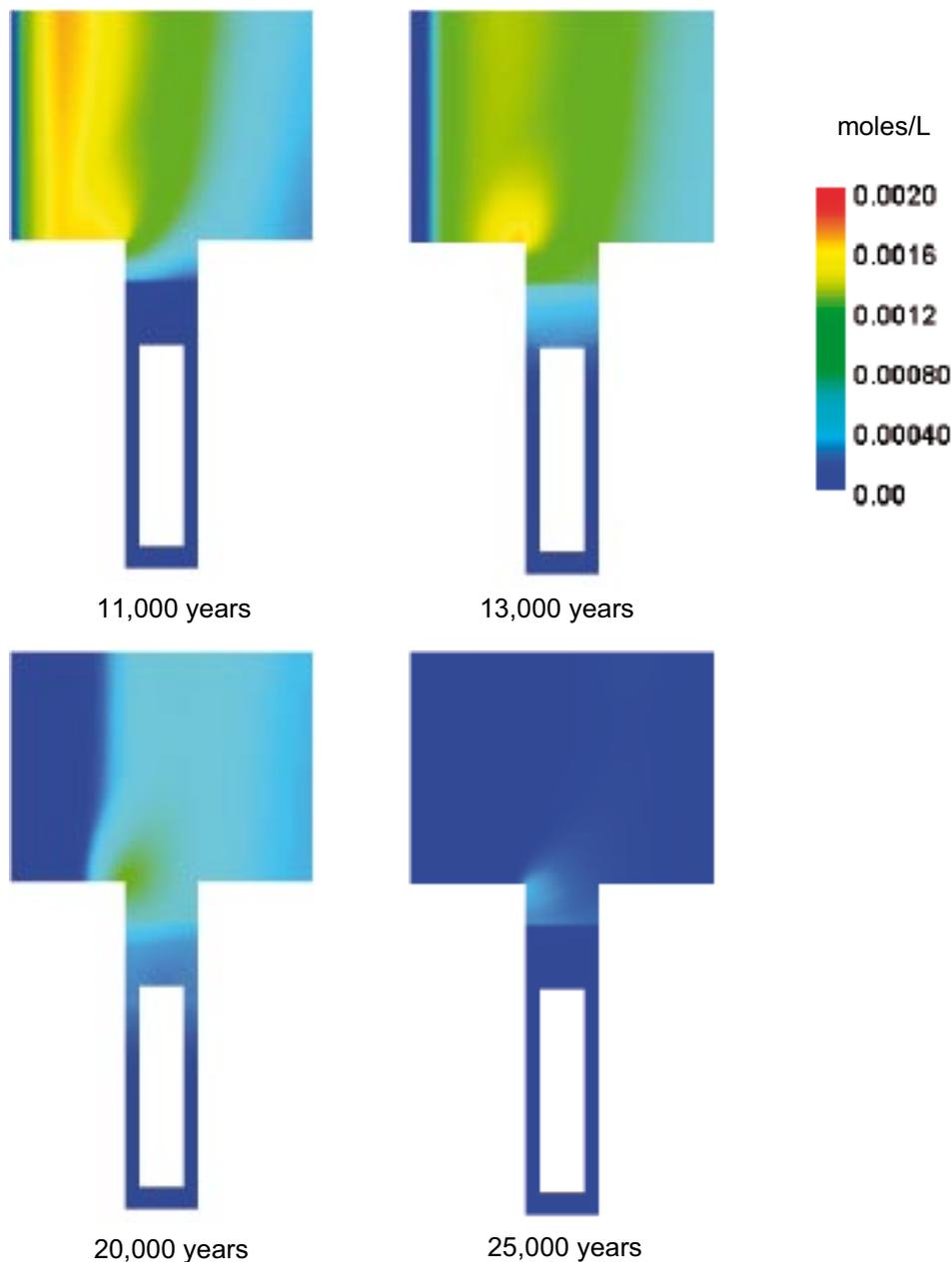
**Figure 5-42.** Predicted precipitation and dissolution of calcite during the intrusion of high-salinity groundwater into the system.
