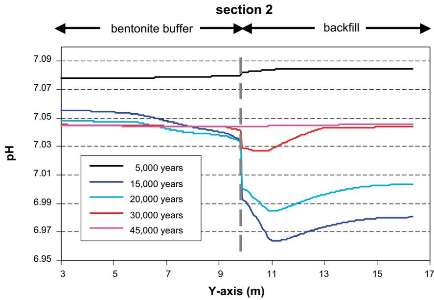
**Figure 5-52.** Graphic showing the predicted evolution of pH after the intrusion of high-salinity groundwater in section 2.
