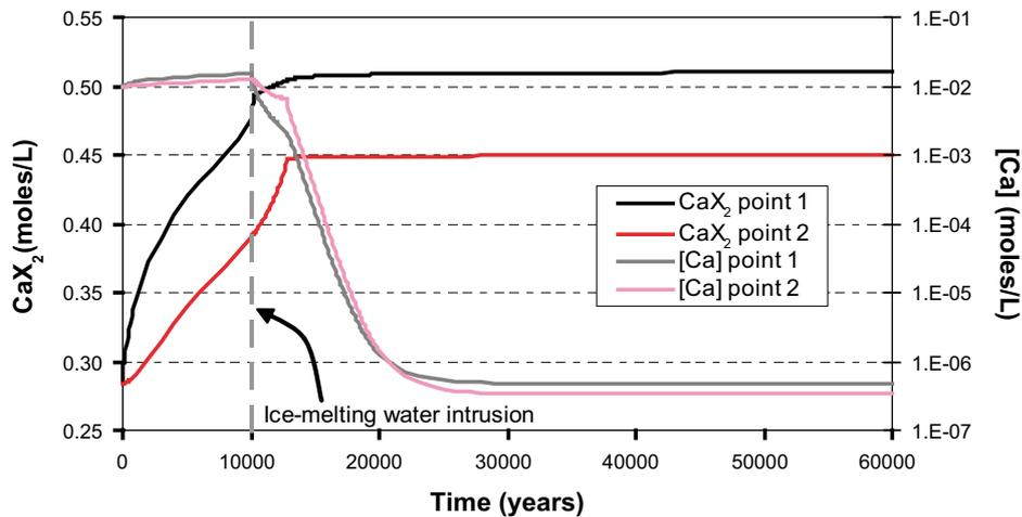
Figure 5-16. Predicted evolution of Ca occupancy in the exchanger and aqueous calcium concentration at two points in the bentonite as shown in Figure 5-10, (1) at the fracture level, and (2) far from the fracture intersection. Note that approximately after ice-melting water intrusion (grey dashed line) the calcium occupancy in the exchanger is predicted to be constant.
