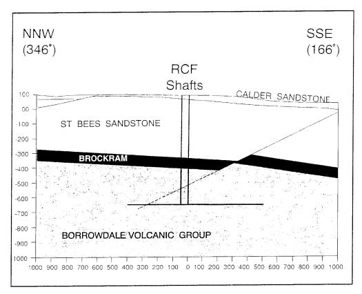
Figure 4.2-2. Projection of RCF, Phases 1 to 3, viewed from WSW.
