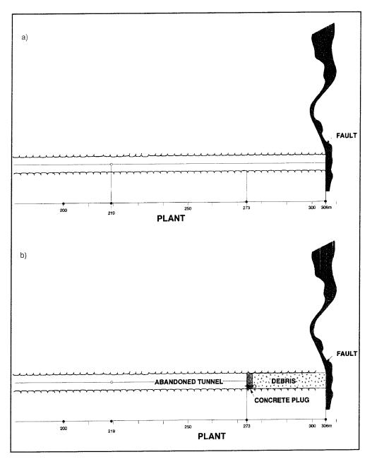
*Figure 2.4-3a.* Normal tunnel excavation without knowledge of the incoming fault. *Figure 2.4-3b.* Complete the plug and abandon the main tunnel.
