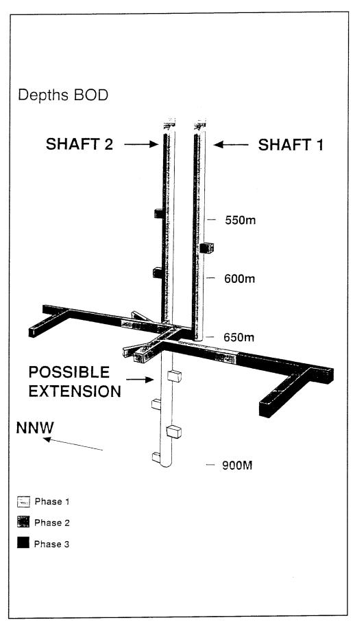
Figure 4.2-5. Schematic design of a rock characterisation facility.
