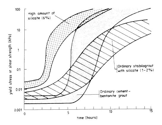
Figure 2.3-3. The effect of silicate.
