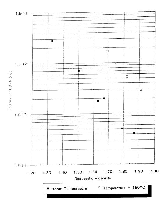
Figure 4.4-5. Hydraulic conductivity (m/s) of FoCa clay versus reduced dry density.
