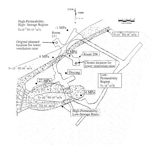
*Figure 2.1-5. Hydraulic transmissivity pattern and normal stress conditions in Fracture Zone 2 beneath 240 Level.*
