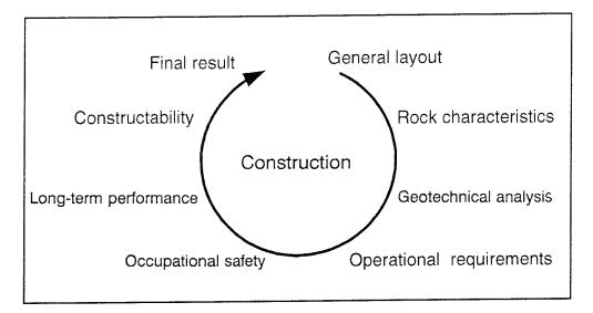
Figure 4.1-3. Factors affecting the construction work.
