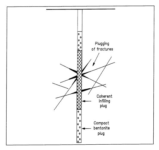
Figure 4.5-2. Tailor-made borehole sealing.
