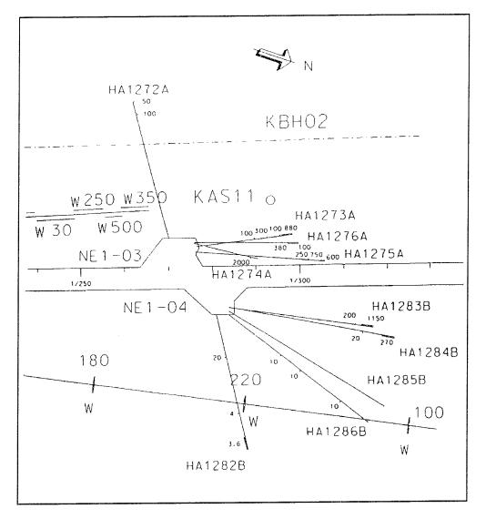
*Figure 2.3-2.* Positions of the percussion boreholes in niches NE1-03 and NE1-04. The figures on the boreholes are the inflow of water in l/min.
