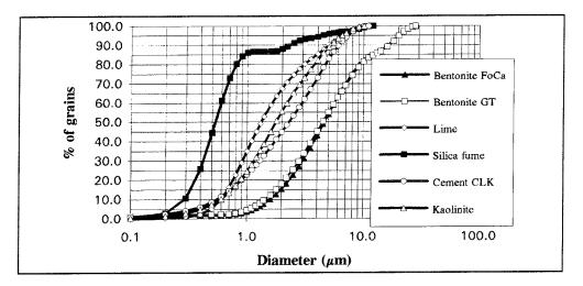
Figure 4.5-3. Grainsize-distribution curves of sealants.
