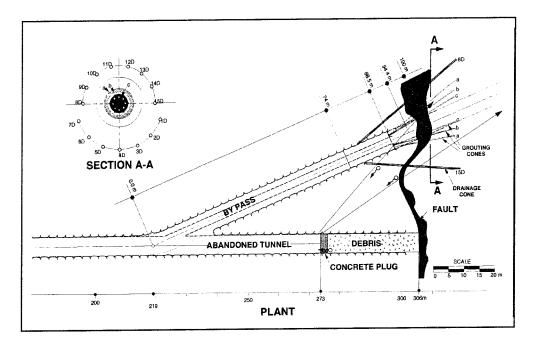
Figure 2.4-5. Complete first three cones of grouting drill holes.
