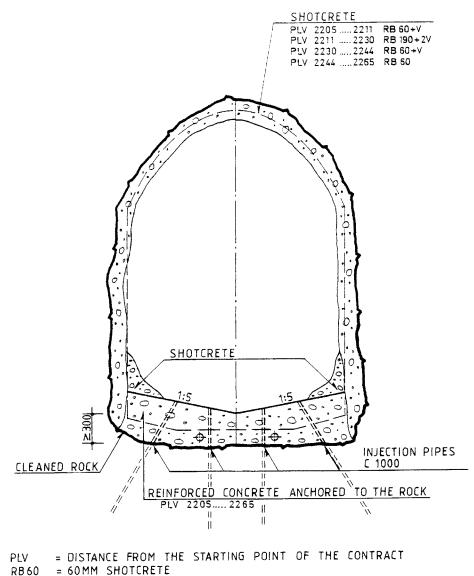
RB60+V = 60MM SHOTCRETE REINFORCED WITH STEEL MESH
