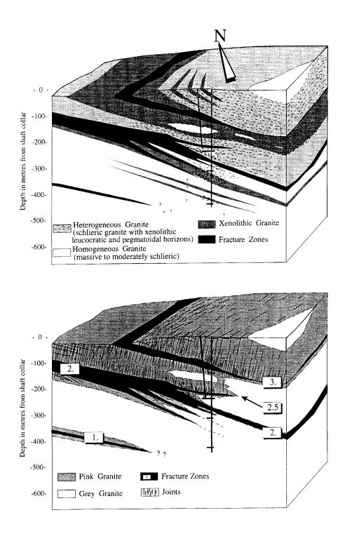
Figure 2.1-2. Geological structure and lithology at the URL /after Everitt et al., 1990/.
