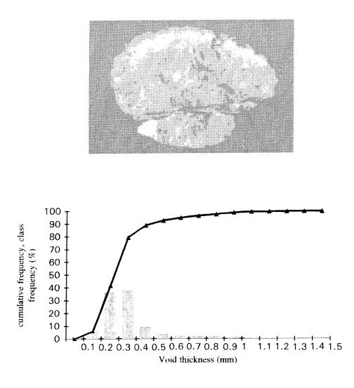
*Figure 4.5-1.* Image of a fracture-wall cast, and the resulting normal and cumulative histograms of void thicknesses in the fracture wall.
