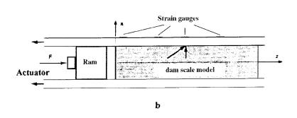
Figure 4.6-3. Clay core dam scale model a) the tube with a rigidity equivalent to the rock mass one b) schematic cross view of the scale model.
