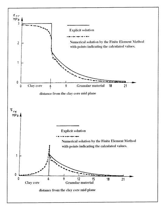
**Figure 4.6-2.** Normal and tagential stress components at the gallery wall as a function of the distance from the clay core dam mid plane.
