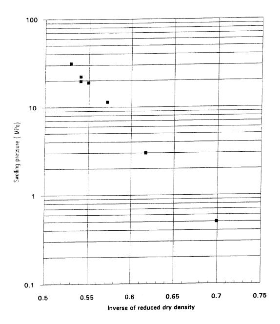
**Figure 4.4-4.** Swelling pressure (MPa) of pure FoCa clay versus inverse of reduced dry density.
