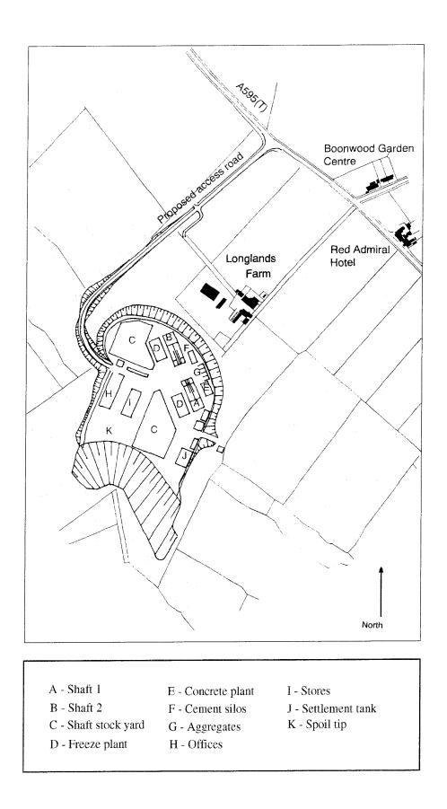
Figure 4.2-4. Preliminary layout of surface development for RCF.
