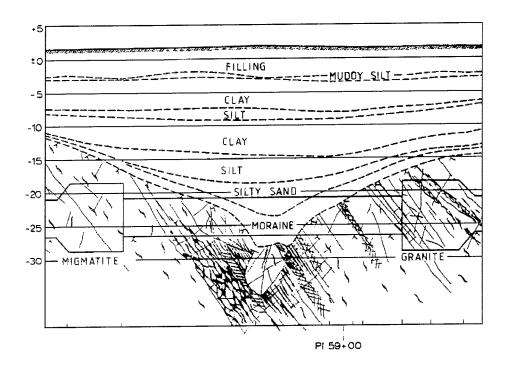
Figure 2.2-6. Soil and rock conditions of the Kluuvi Cleft /Hartikainen et al., 1978/.
