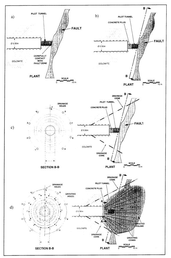
Figure 2.4-6a. Final phase. First contact with fault zone. Figure 2.4-6b. Final phase. Installation of concrete plug. Figure 2.4-6c. Final phase. Installation of drainage cone. Figure 2.4-6d. Final phase. Complete grouting volume.
