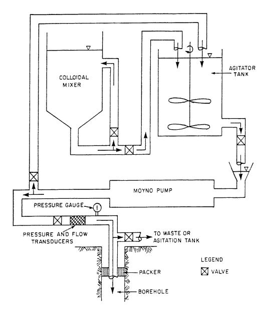
Figure 4.3-4. Schematic arrangement of grouting plant.
