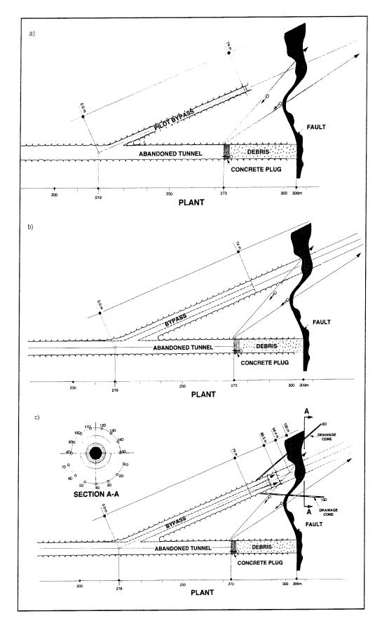
Figure 2.4-4a. Start of the pilot bypass tunnel. Figure 24-4b. Enlargement of the bypass tunnel. Figure 2.4-4c. Complete drainage cone.
