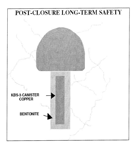
SKB 91 ... "shows that a repository deep in Swedish crystalline basement rock with engineered barriers possessing long-term stability fulfils the safety requirements proposed by the Swedish authorities with ample margin.
