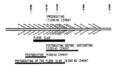
Figure 2.2-3. Sea Sewer. Grouted area and number of pregrouting rings.
