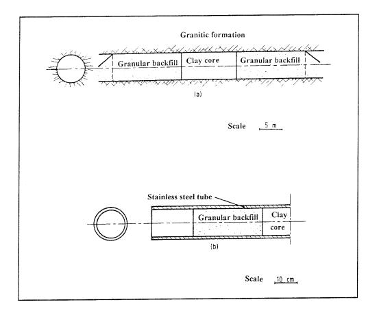
Figure 4.6-1. Clay core dam schematic layout and its scale model a) dimensions issued from stability analysis, b) scale model implaced in a stainless steel tube.
