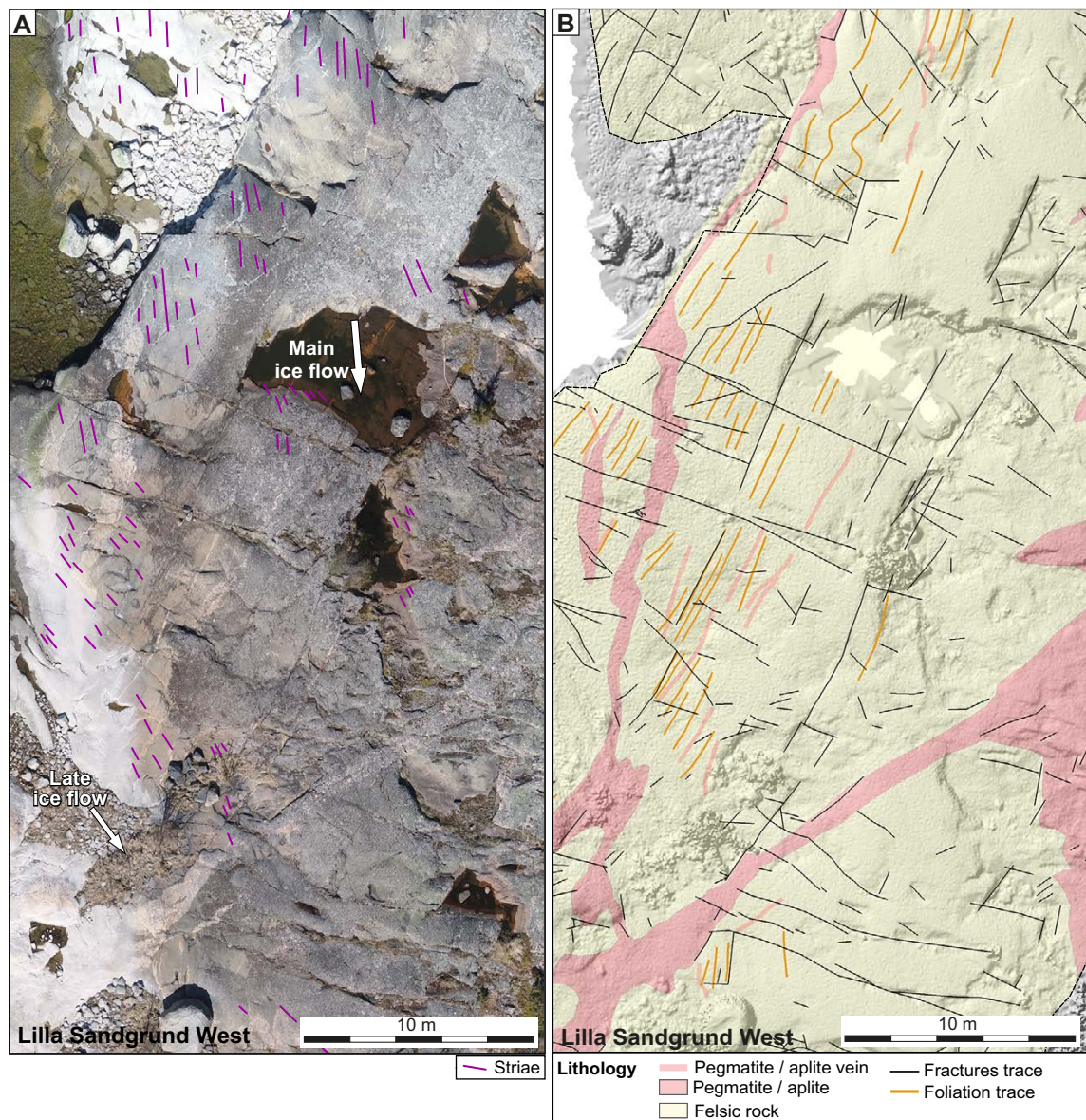
Figure 5-10. Drone-acquired imagery and mapping for Lilla Sandgrund West. A. Orthophoto, with striae traces. B. Lithology and fracture traces; hillshade from DSM as background.
