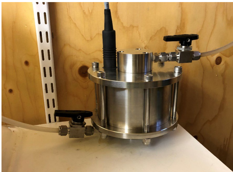
Figure 3-5. Fluorescence detector GGUN- FL30 connected for online measurement.
