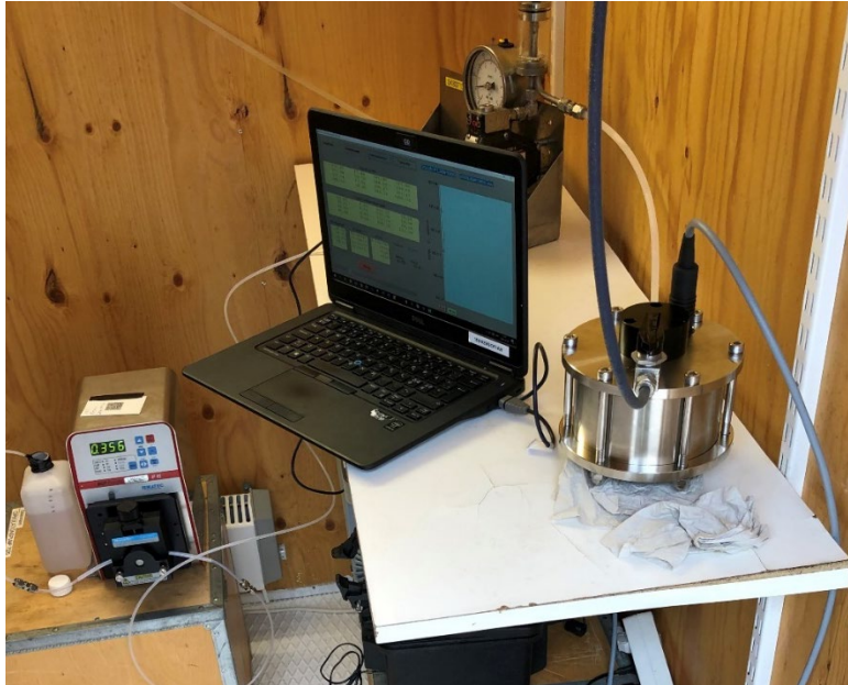
Figure 3-4. All equipment during injection. Pump for tracer injection to the left, circulation unit in the back, fluorescence detector in the front connected to the logger under the bench. The logger is during injection connected to the computer, which makes it possible to follow the concentration in real time.
