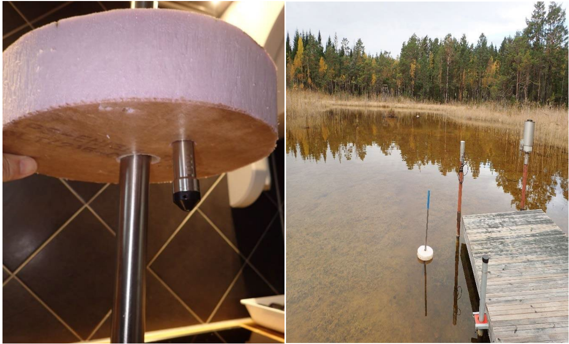
Figure 2-1 Setup for measurement of water temperature at a specific depth. A foam block is used to float the sensor as well as protect it from direct solar radiation. A stake is then used to fix the setup in location and allow the sensor to float up or down as water levels change.
