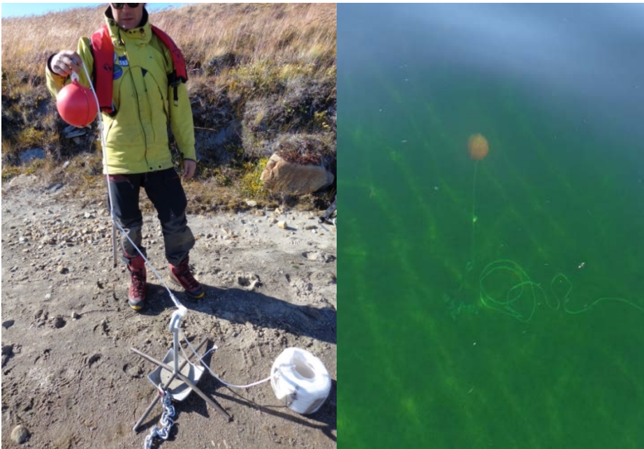
Figure 9. Pressure transducer measuring the water level fluctuation in TBL.
