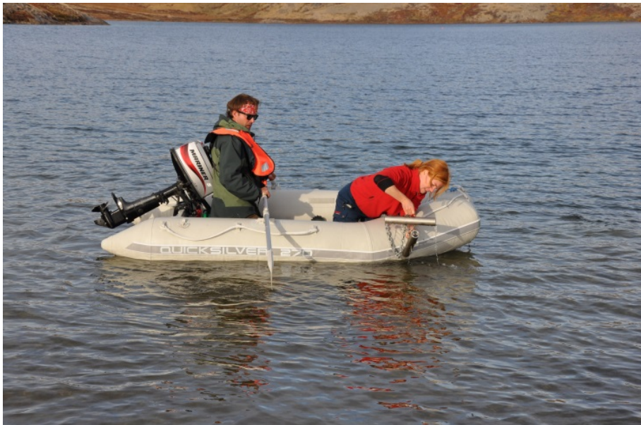
Figure 8. Installation of the pressure transducer measuring the water level fluctuation in TBL.
