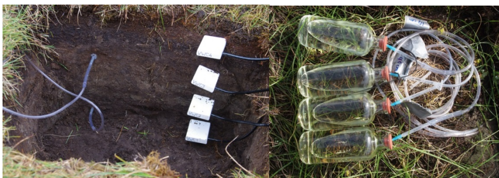
Figure 15. Lysimeter and TDR installations in the active layer. To the right: lysimeter flasks with soil water ready to collect.
