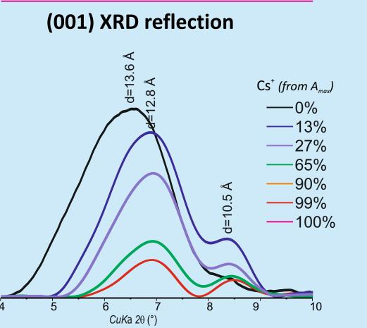
The mechanism of the cesium adsorption on montmorillonite after a thermochemical impact differs significantly from the natural montmorillonite. The main reason appears to be related to changes of the layer charge and a partial interlayer protonation. Cesium substitutes oxonium than Ca and Mg. The total amount of the adsorbed cesium is determined by capacitive abilities of montmorillonite and thus is reduced after a long-term treatment with nitric acid solutions.
