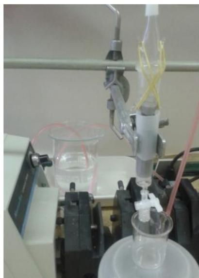
Fig. 1: The dynamic column experiment.
