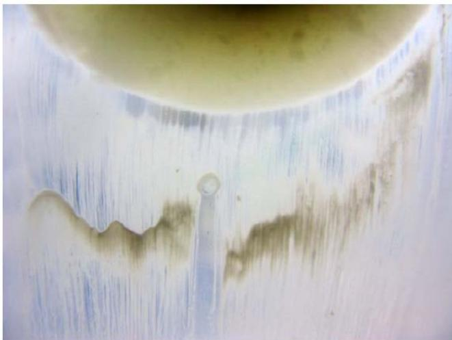
Figure 2. Close-up picture of sedimenting agglomerates in de-ionised water. The cylindrical region is 2 cm in diameter. Figure 59 in (5).
