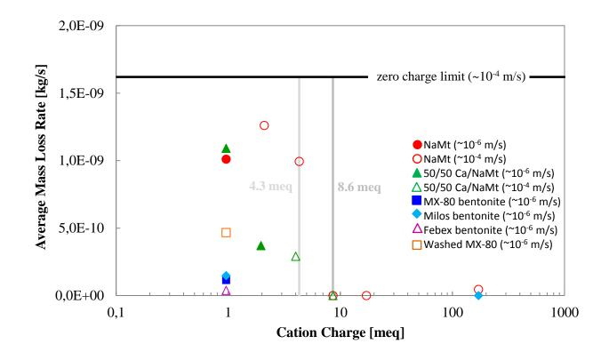
☐ Average mass loss rates for various sample materials from horizontal, 1 mm aperture, artificial fracture tests as a function of cation charge equivalents for solutions flowing through the fracture systems.
