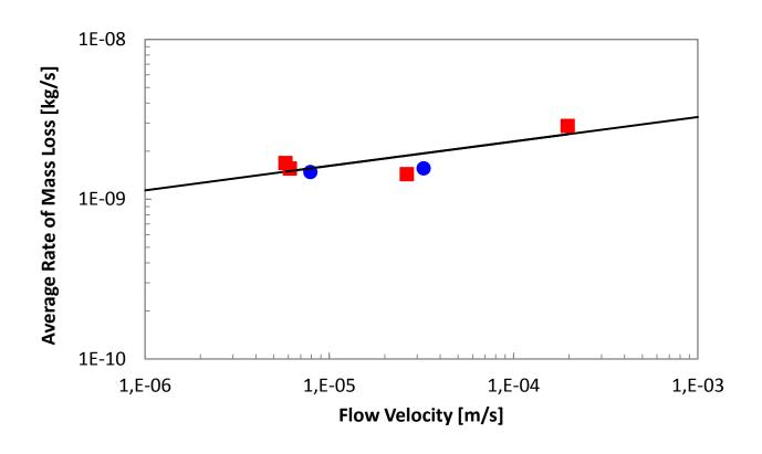
☐ Overall mass loss rates for (maximal) horizontal, artificial fracture tests are reasonably well-correlated to flow velocity.
