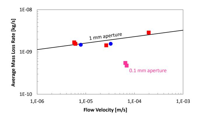
☐ Consistent with surface-area controlling effect on mass loss.
