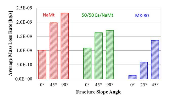
☐ In every case conducting tests, that in all other respects are identical, at larger slope angles leads to increased mass loss rates.
