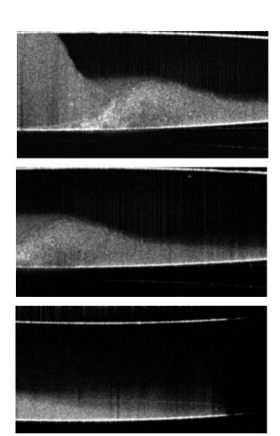
Aggregation and sedimentation of the eroding material occurs downstream of the source; some fraction of the initially eroded mass becomes sedimented and will not be readily transported out of the near-field.
