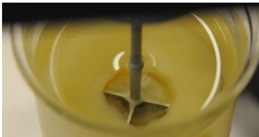
Figure 2. Ku-mmt, 20g/l in 20 mM NaCl(aq) after a yield stress measurement.
