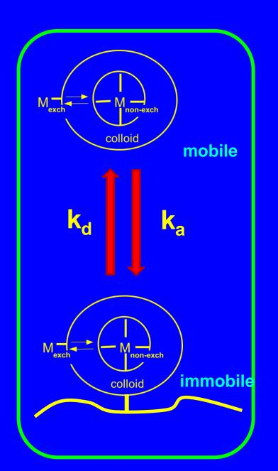
Interaction of the colloid with a surface will affect transport. For a simple first order attachment/dissociation mechanism:
