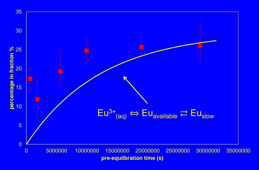
Not possible to simulate data very well with just a single slow fraction. The 1 day expt also has a different dissociation rate.
