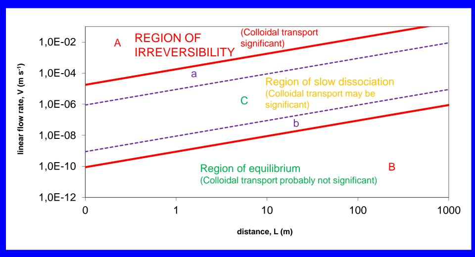
Changing the rate constant makes a significant difference to the region where colloidal transport may be significant.
