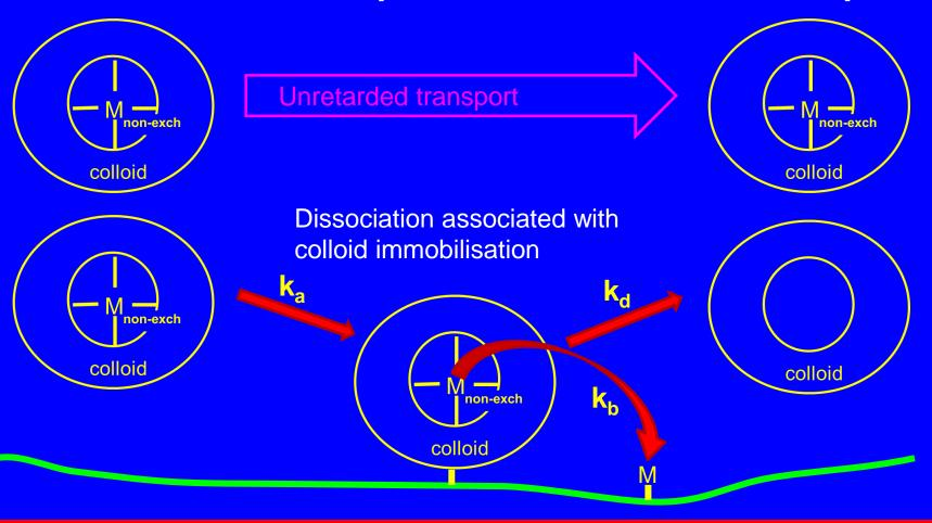
$$D_{M} = \frac{k_{b}}{V}L \Big|_{D_{C} \to 0} \qquad D_{C} \text{ increasing} \qquad D_{M}^{eff} = \frac{k_{b}}{V}L(1+K_{C})\Big|_{D_{C} \to \infty}$$
