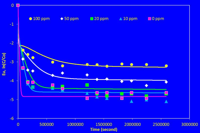
Significant chemical fractionation required in order to explain data: minor (30%) component with higher (x130) binding strength.
