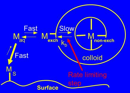
$$\begin{array}{ccc} & k_b \\ M_{exch} & \xleftarrow{\longleftarrow} & M_{non-exch} \\ \\ \frac{d[M_{non-exch}]}{dt} & = & k_f[M_{exch}] - k_b[M_{non-exch}] \end{array}$$
