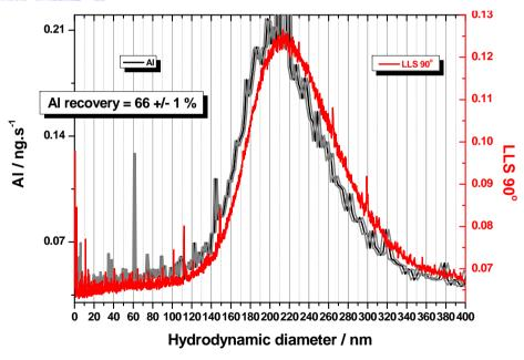
Colloidal fraction + huge aggregates found in a 10 y old FEBEX bentonite colloid solution stored in a brown PET,  $pH_f$  8.0
