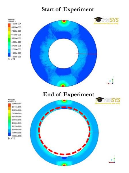
SKB TR-10-64 (Bentonite erosion model)
