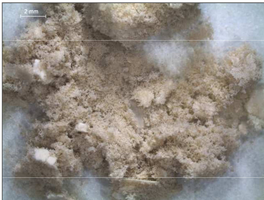
Bentonite after lyophilization – stereomicroscope pictures
