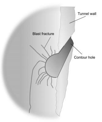
Fig. 3. Part of an investigation slot surface showing blast fractures near a blast hole halfpipe. Hole diameter is 48 mm.
