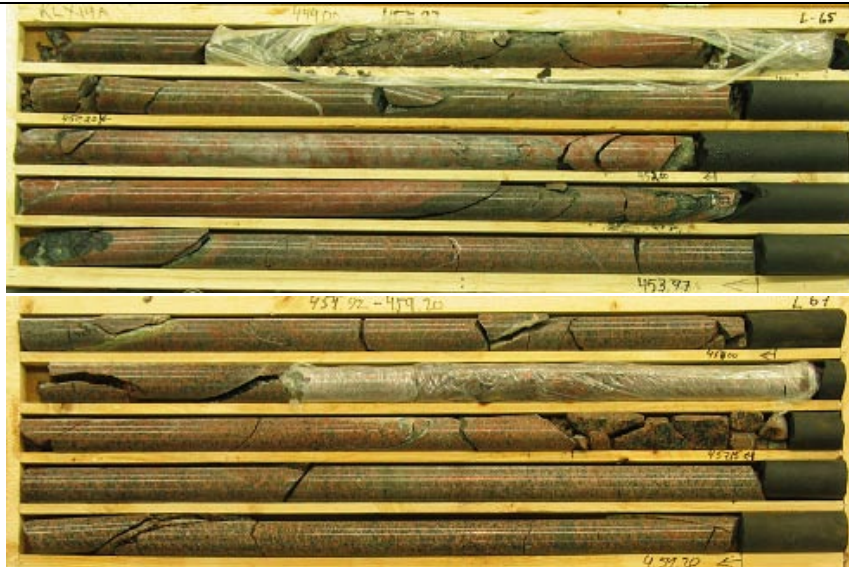
KLX19A 449-459 m borehole length. Part of DZ4, including part of one (of two) core zone 448.0-457.2 m.
