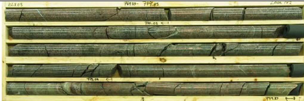
KLX03A 769.39-774.83 m borehole length. Part of DZ1b including part of core zone 767.50-774.60 m.
