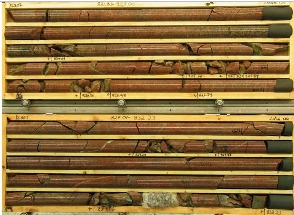
KLX07A, 821.83-832.23 m borehole length. Part of DZ13, no defined core zone.
