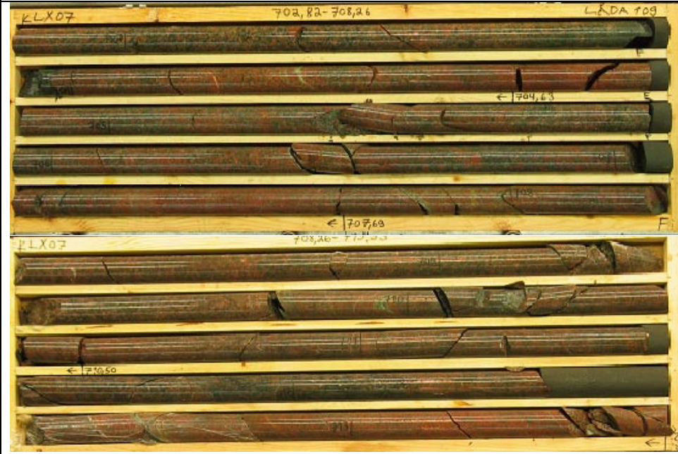
KLX07A 702.82-713.53 m borehole length. Part of DZ11 (no defined core zone)
