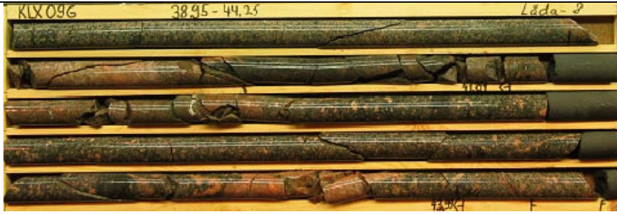
KLX09G 38.95-44.25 m borehole length. Part of DZ1 including one (40.38-41.50 m) of two core zones.
