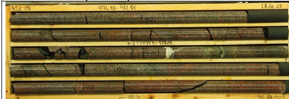
KLX08A 476.48-481.84 m borehole length. Part of DZ7 including core zone 478.3-479.5 m. Note ZSMEW946A is interpreted as a sequence of such structures.
