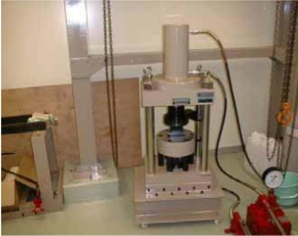
*Figure B-3. Compression molding machine used to create buffer blocks for the BORE-SHEAR test specimens.*
